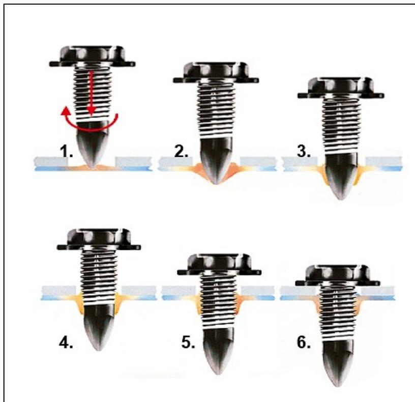
*Fig. 1.14 Fasi Flow-drill Screwdriving*
