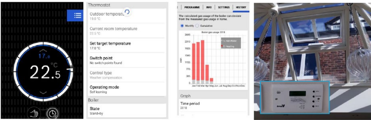
Fig.20 Smart controls for the heating and hot water - Automatic smart conservatory top vent (SRI project)
