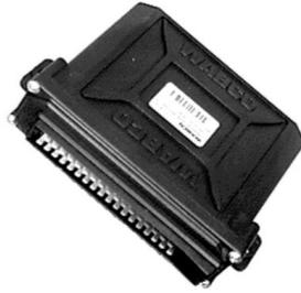
**Figura 2.5:** Centralina Electronically Controlled Air Suspension
