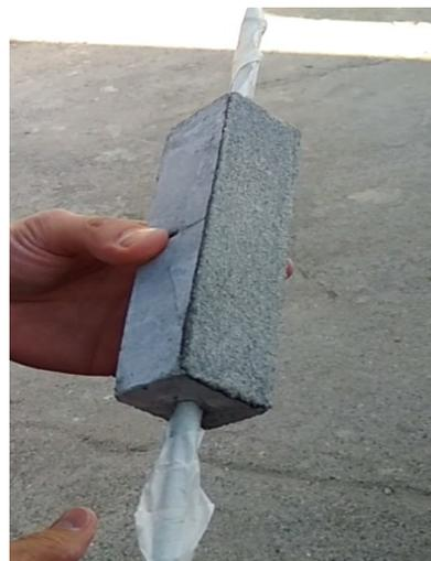
Supporto prova crack-bridging
