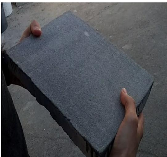
Supporto prova crack-bridging STATICO
