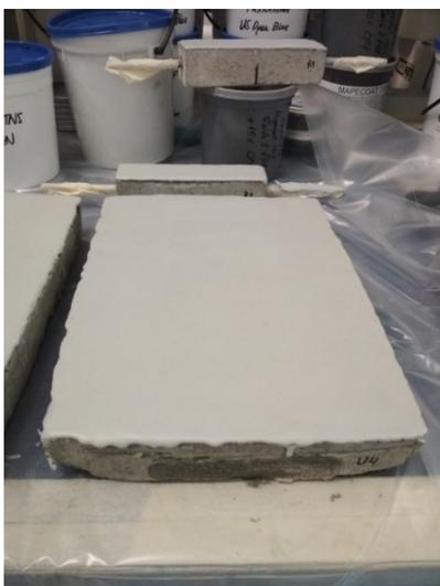
Supporto prova crack-bridging
