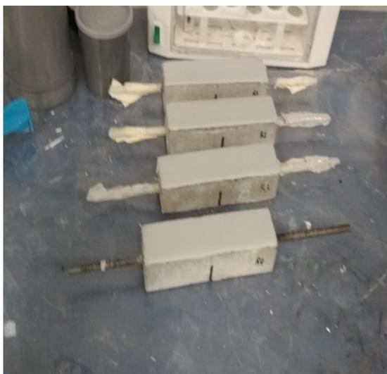
Supporto prova crack-bridging
