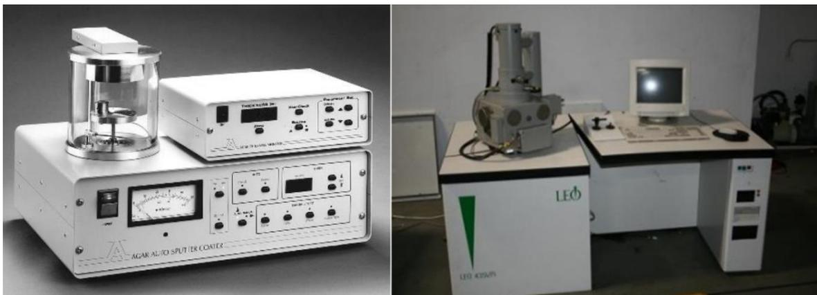
**Figura 18: Agar Auto Sputter Coater e LEO 435VP SEM**
