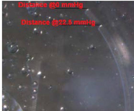
Figure 3.10: The position of the fluid-air interface when pressure assumes the smallest value, 0 mmHg, and the greater value 22,5 mmHg regarding the pressure range tested. The interface totally moves about 0,912 mm [32].
