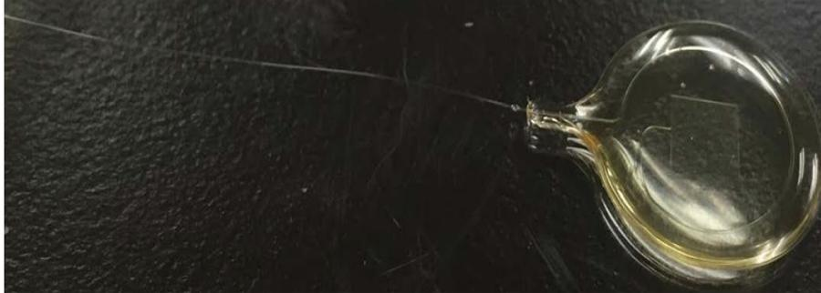
Figure 3.7: Prototype of the intracranial pressure sensor [32]
