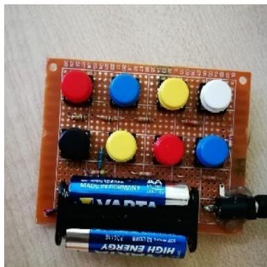
Figure 6.6: Pushbutton pad; each button corresponds to a different voltage value.
