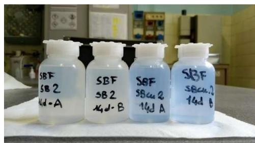
Figure 4.33: SBCu glasses after 14 days in SBF
