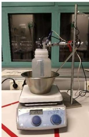
Figure 3.14: Set-up for preparation of SBF solution
