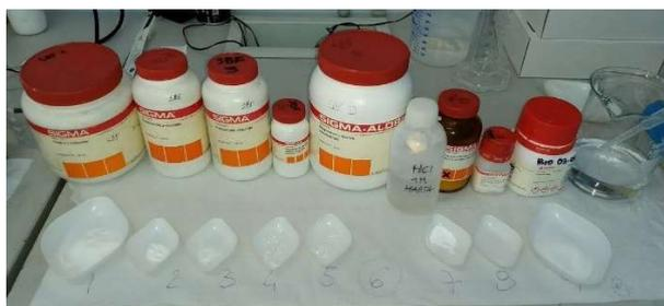
Figure 3.5: Chemical reagents for preparation of SBF solution
