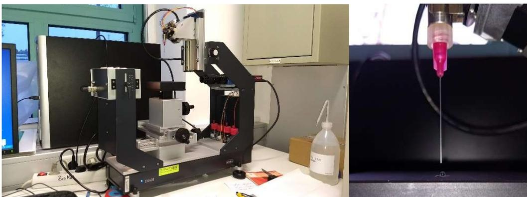
*Figure 3.13: Contact angle measurements set-up*
