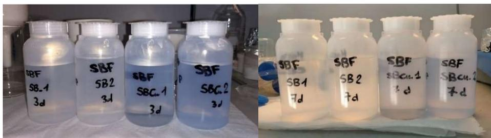
Figure 4.32: SBCu glasses after 3 days (left) and 7 days (right) in SBF
