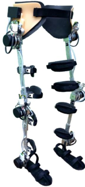
Figure 2.1: The H2 exoskeleton[16], a bilateral hip, knee and ankle active joint rehabilitation device.
