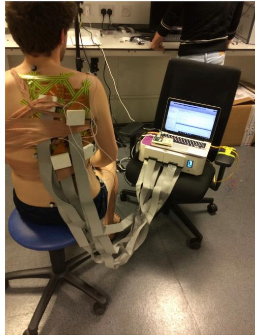
(b) The entire setup connected setup. It is clearly visible from this picture the complexity of the setup. The acquisition system is also visible and it is above a wheeled chair to allow the researcher to follow the subject during the execution of the tasks.
