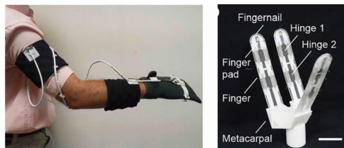
Figure 1-22 The wrist exoskeleton [35] and the Soft gripper [34]
