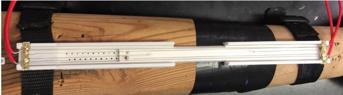
Figure 2-9 SMA wire module as at the end of the prototyping process. This module contains all the needed SMA wires which are actuated with the red current cables coming from the SMA driver.
