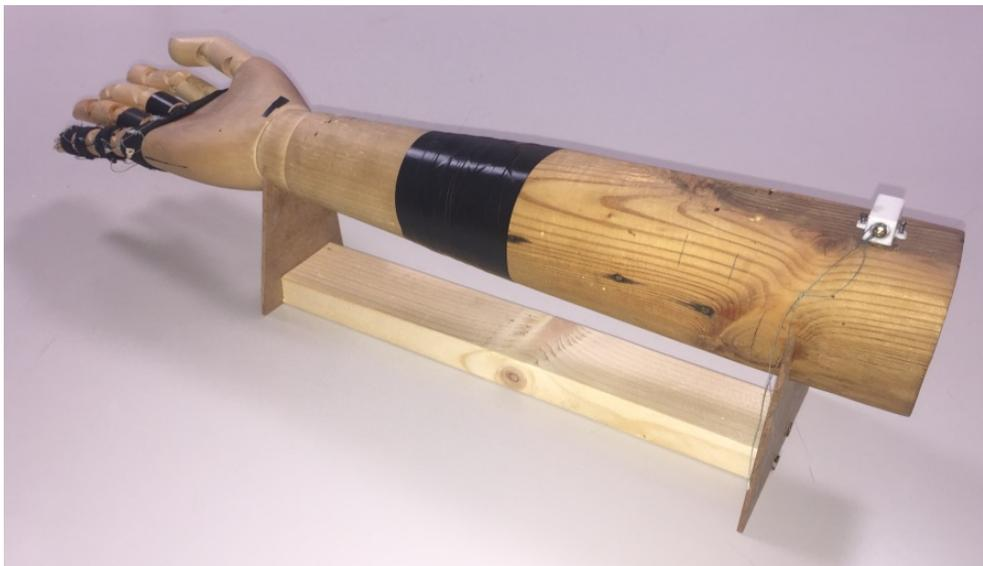
Figure 4-1 The wooden armrest construction built to obtain a fixed and stable position during the measurements
