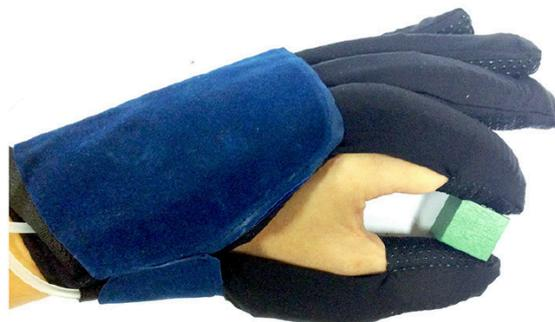
Figure 1-11 Pneumatic Soft robotic glove by Yap [20]
