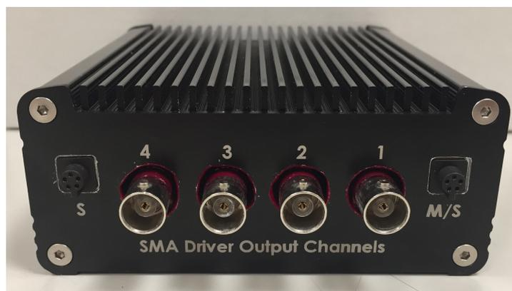
Figure 2-8 SMA driver unit, four cables can be connected to the channels to actuate the SMA wire modules.
