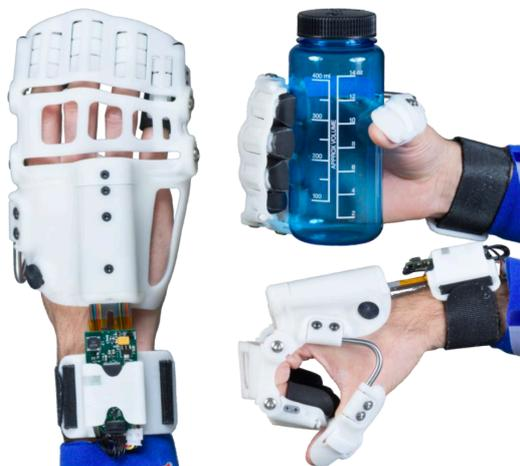
Figure 1-18 Prototype of Vanderbilt hand exoskeleton [29]
