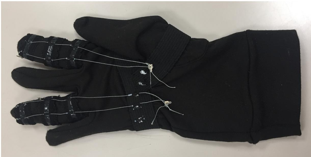
Figure 3-15 Final glove design with tendon system. Kevlar wires pass through tubes which are attached to elastic straps around the phalanges. The SMA wire can be hooked onto the small metallic part at the end of the tendon.
