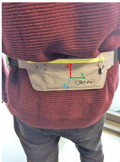
Figure 3.1: Smartphone position and axis orientation adopted during the examination.
