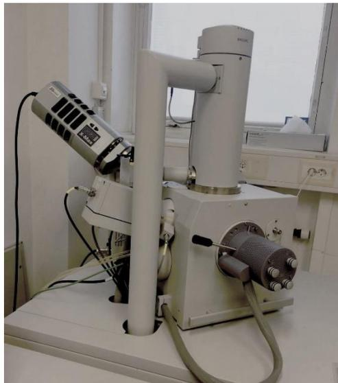
Figure 5.4 . SEM used during this study
