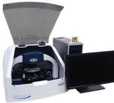
Figure 5.6 . Bruker Dektak XT Precision Profilometer
