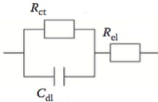
Figure 20 Simplest case of equivalent circuit
