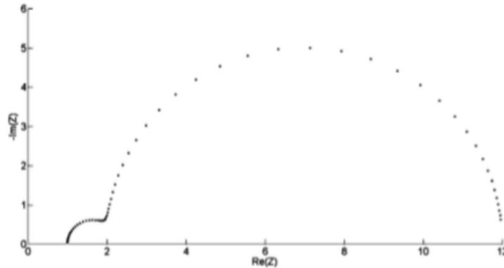
Figure 25 Nyquist Plot for  $R_1 = R_2 = 1\Omega$ ,  $R_3 = 10\Omega$  and  $C_1 = 0.01\text{ F}$ ,  $C_2 = 0.1\text{ F}$  for a frequency range of 10 mHz-100kHz.
