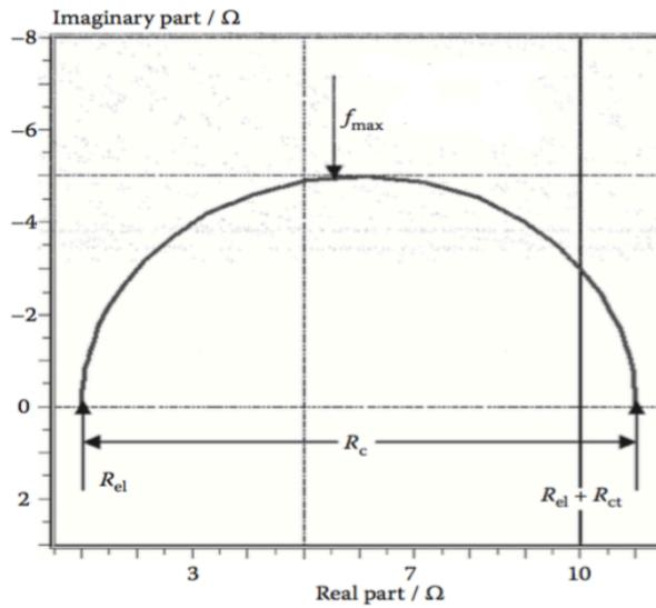
Figure 21 Nyquist Plot for the equivalent circuit of Figure 20, frequency range: 10mHz-10kHz
