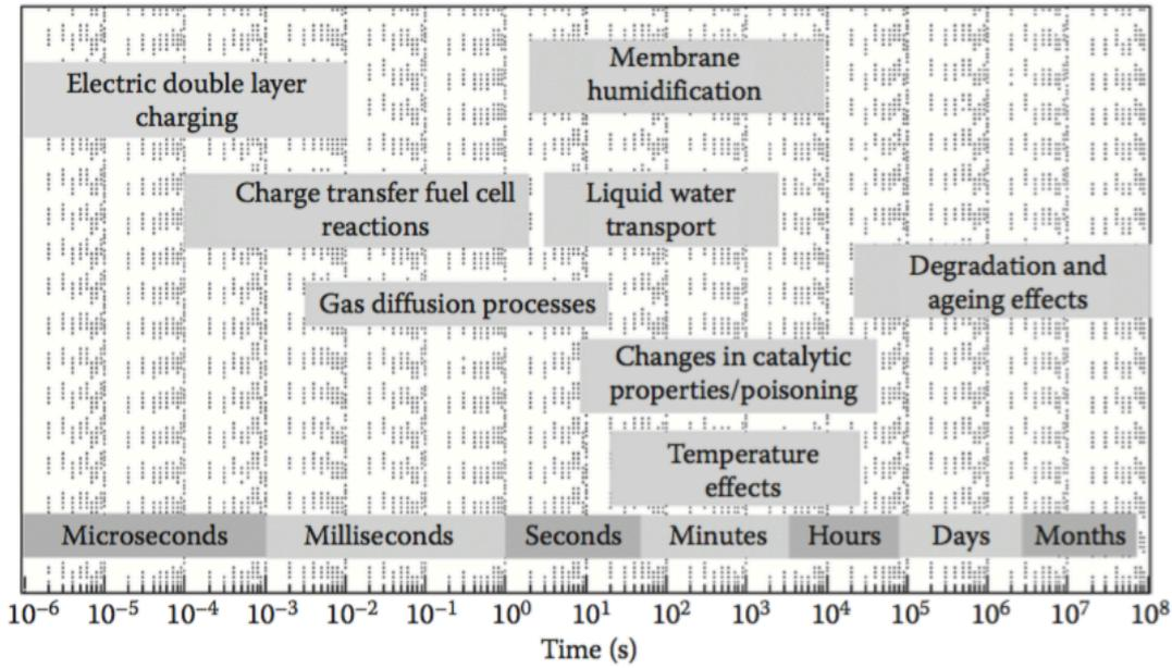
Figure 4 Representation of the many frequencies characterizing each fuel cell reactions
