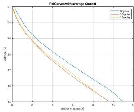
Figure 11 Polarization Curves referring to the first testing day (15<sup>th</sup> of March)
