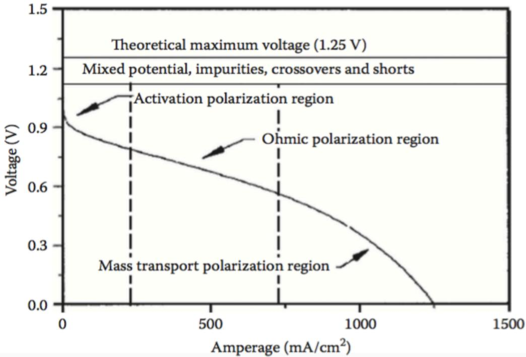
Figure 2. A typical polarization curve for a PEMFC. (Reproduced from Journal of Power Sources, 70, Lee, J.H., Lalk, T.R., and Appleby, A.J., Modeling electrochemical performance in large scale proton exchange membrane fuel cell stacks.)
