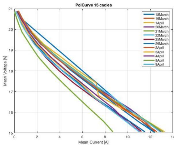
Figure 16 Polarization Curves referring to the whole duration of the tests (18<sup>th</sup> of March until 9<sup>th</sup> of April) after 15 cycles
