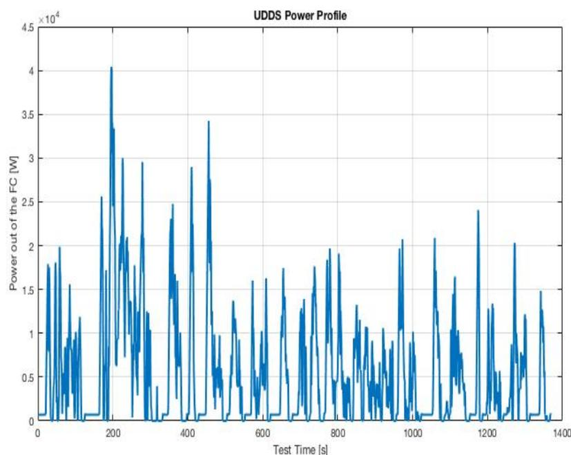
*Figure 8 Power out of the Fuel Cell correspondent to the UDDS*
