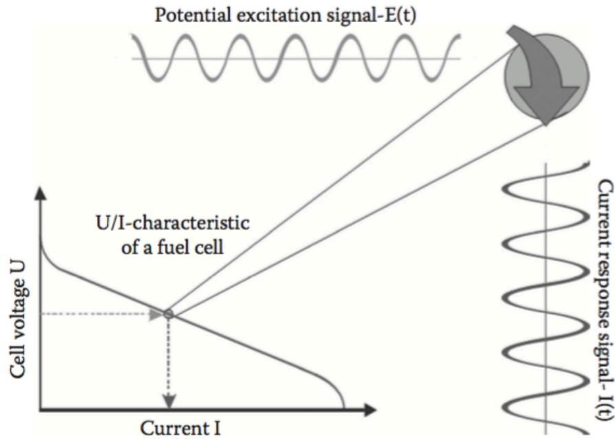
Figure 3 Representation of EIS applied to a fuel cell
