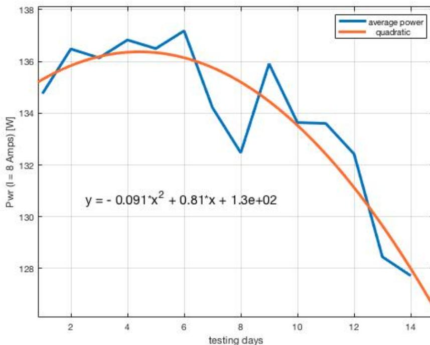
Figure 30 Average power distribution corresponding to a fixed value of current as function of the number of the testing days.
