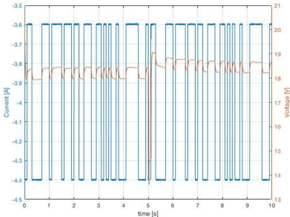
*Figure 17 Current following the PRBS signal and the resulting voltage imposed to the fuel cell before starting with the cycles the 18<sup>th</sup> of March.*
