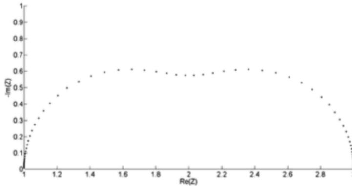
Figure 23 Nyquist Plot for  $R_1 = R_2 = R_3 = 1 \Omega$ , and  $C_1 = 0.01 F$ ,  $C_2 = 0.1 F$  for a frequency range of 10 mHz-100kHz
