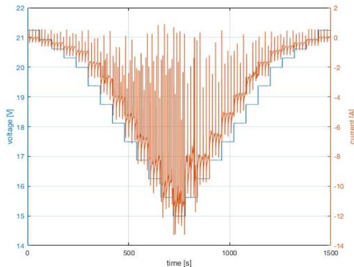
Figure 10 Example of the data necessary to build the polarization curve.
