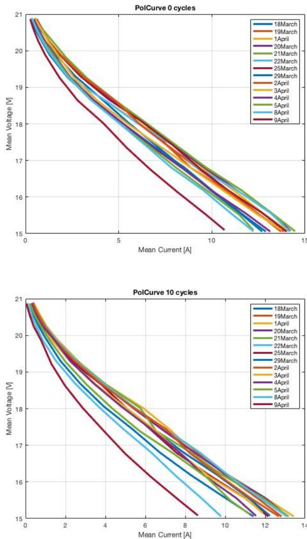
Figure 15 Polarization Curves referring to the whole duration of the tests (18<sup>th</sup> of March until 9<sup>th</sup> of April) after 0 cycles (upper graph) and 10 cycles (down)
