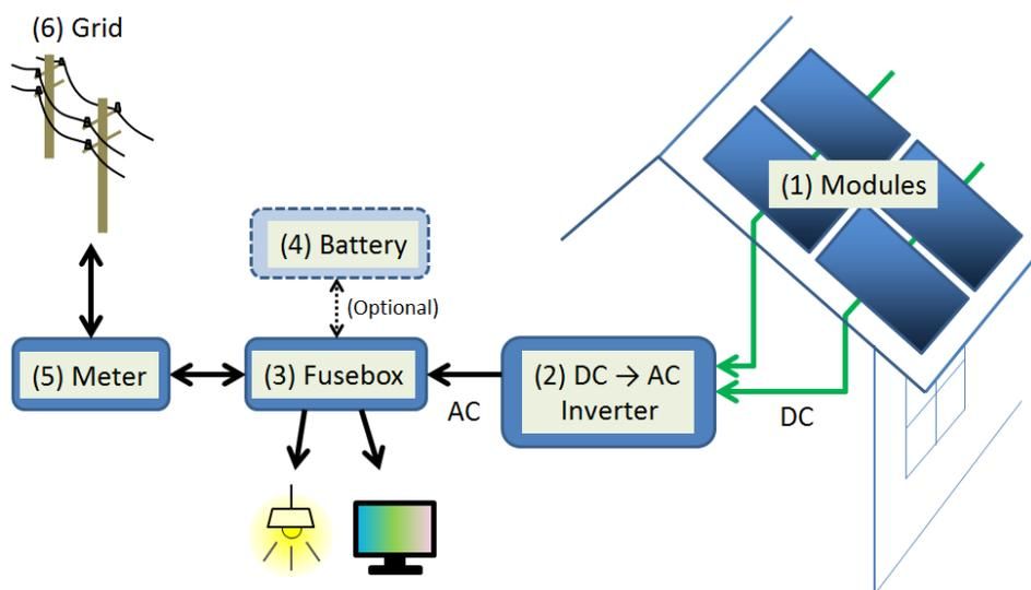
Figure 2 – Scheme of a residential photovoltaic system
