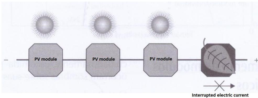
Figure 8 – PV modules with shading in one cell without bypass diode (VILLALVA, 2015)
