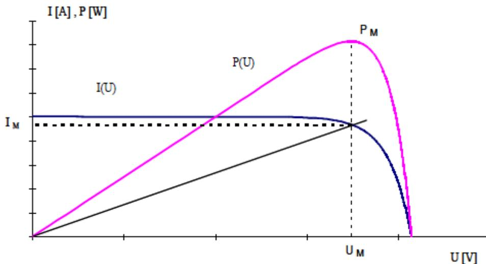
Figure 6 – I-V characteristic curve and correspondent power output (SPERTINO, 2016)
