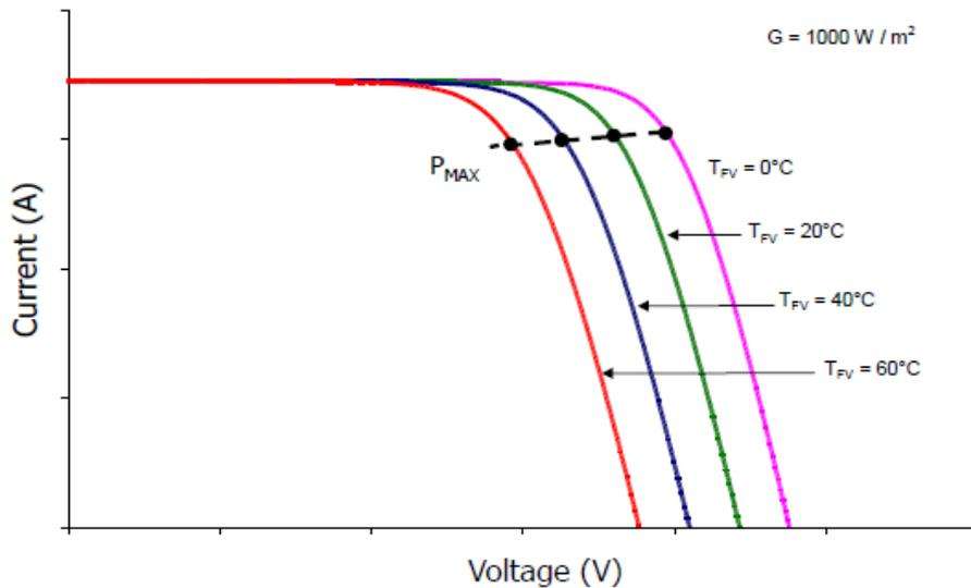
Figure 10 – I-V curve as a function of temperature (SPERTINO, 2016)
