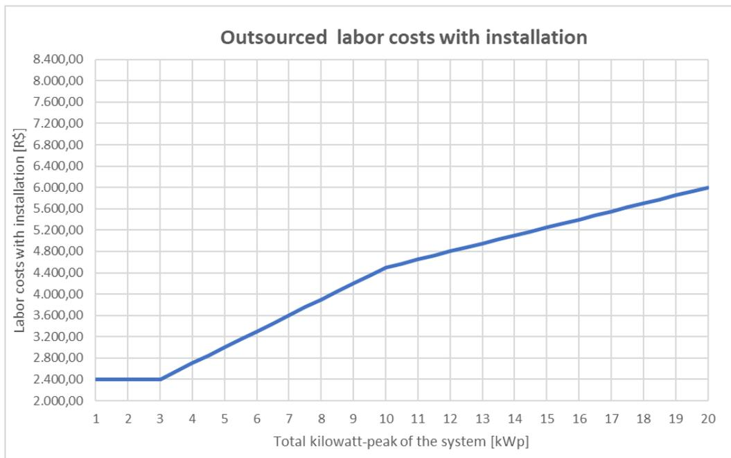
Figure 19 – Outsourced labor costs with installation (Solstar, 2019)
