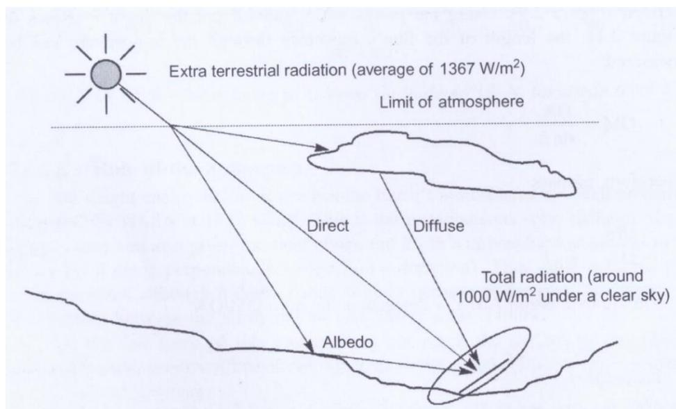
Figure 1 – Components of Solar Radiation on the ground (VILLOZ & LABOURET, 2010)
