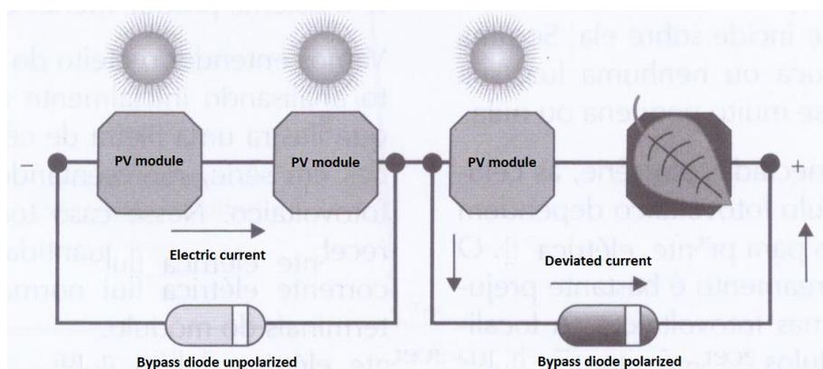
Figure 9 – PV modules with shading in one cell with bypass diode (VILLALVA, 2015)
