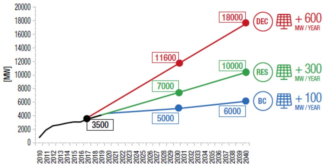
FIG: 2.4. Installed solar capacity per scenario in Belgium [7]
