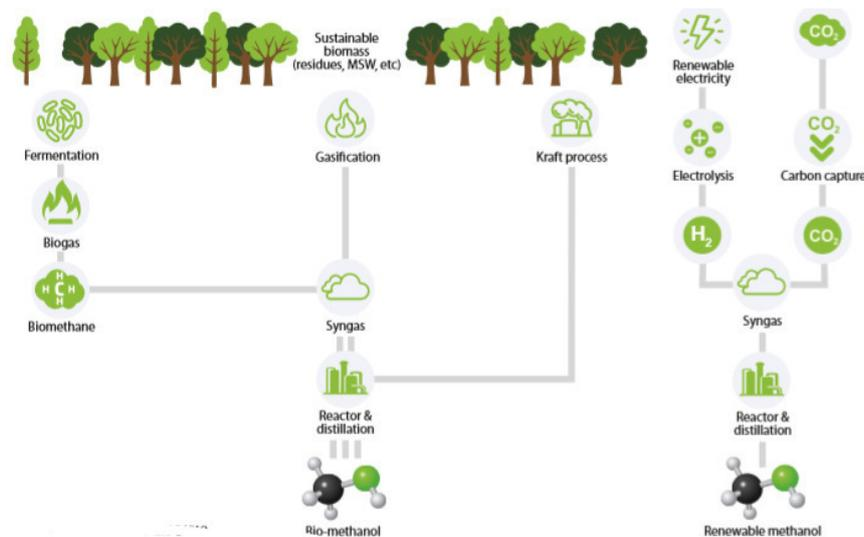
**FIG: 3.2.** Renewable methanol production processes from different feedstocks [25]
