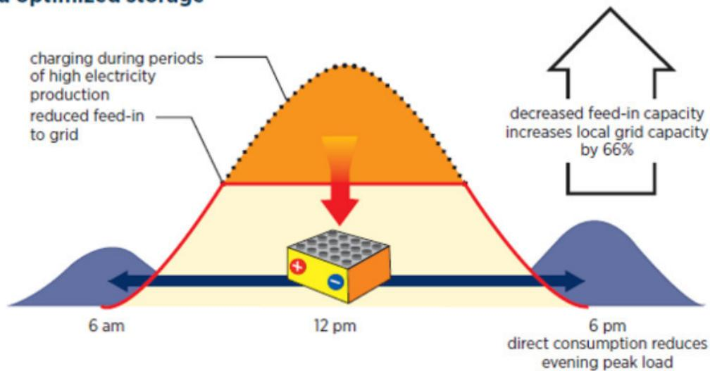
FIG: 3.8. Battery storage shaving peaks while increasing self-consumption[33]
