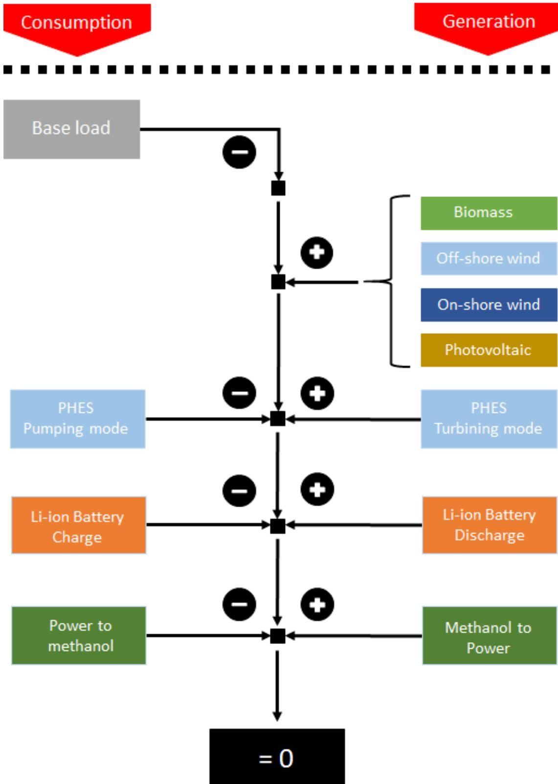
FIG: A.3. Algorithm used in the for-loop
