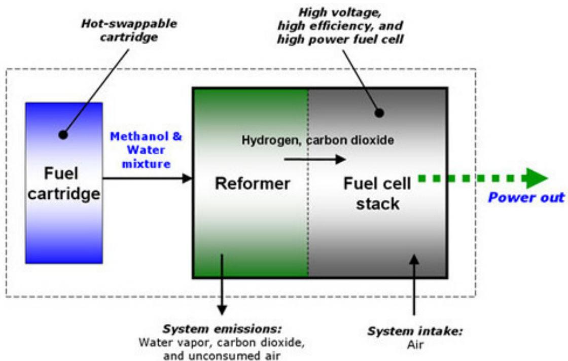
FIG: 3.4. Operation principle of RMFC [62]
