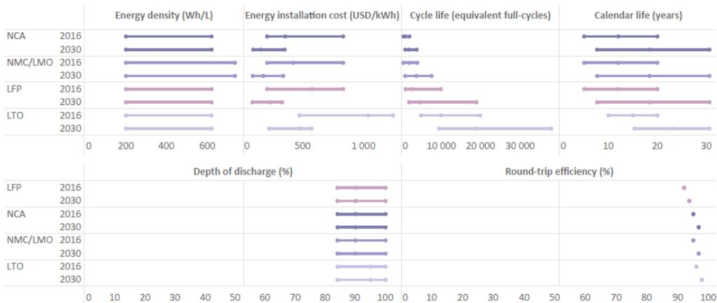
FIG: 3.10. Summary of the different types of Li-ion battery properties [3]
