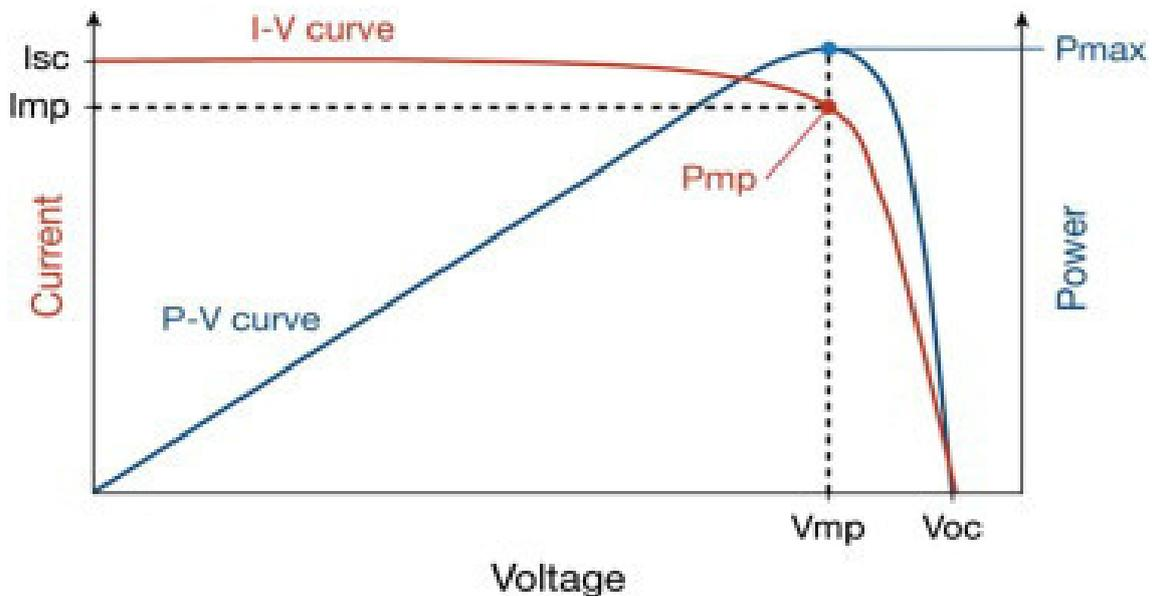
**FIG: 2.5.** Characteristic curves of a typical PV module in certain solar irradiance and temperature. [32]
