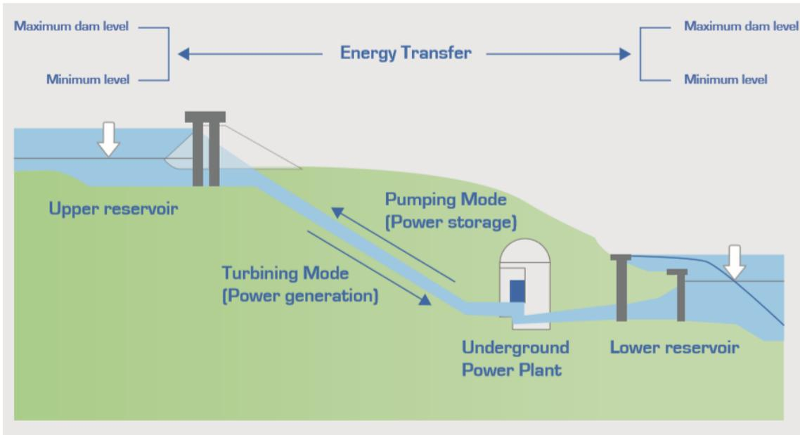
**FIG: 3.6.** Schematic of pumped hydro storage system [4]
