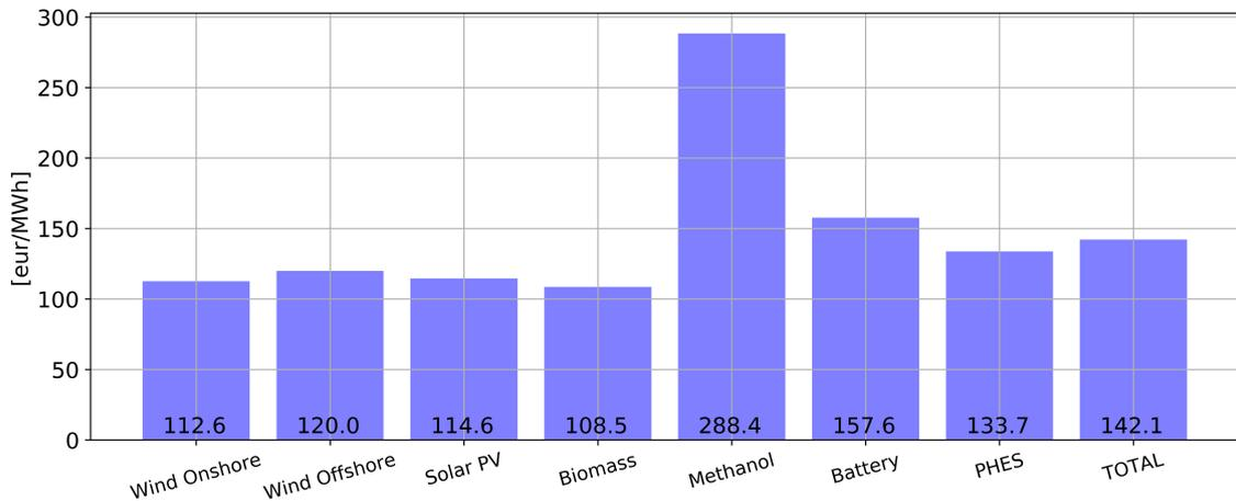
**FIG: 5.12.** Levelized Cost Of Electricity for each technology - base case
