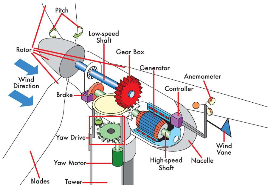
FIG: 2.2. A visual representation of the machinery components [52]
