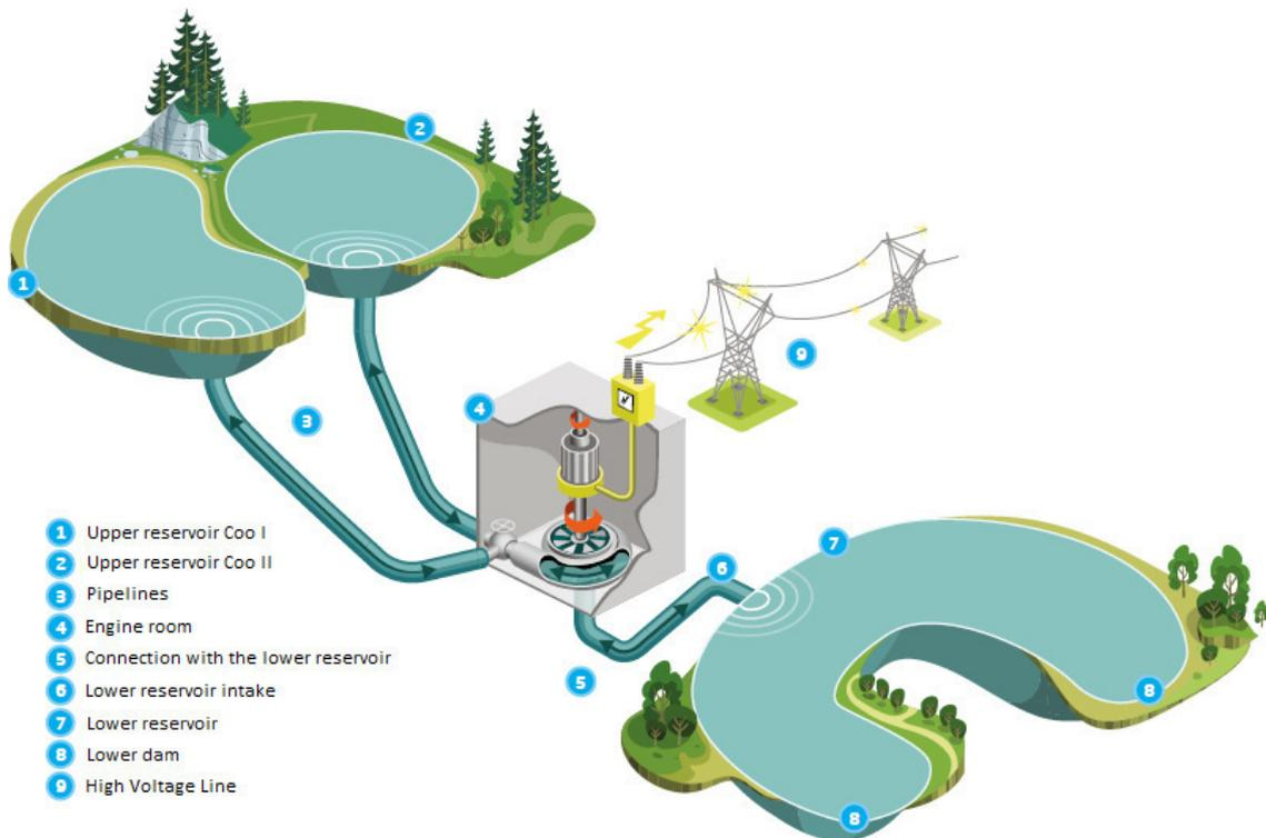
FIG: 3.7. Scheme of the "Centrale de Coo Trois-Ponts" [8]
