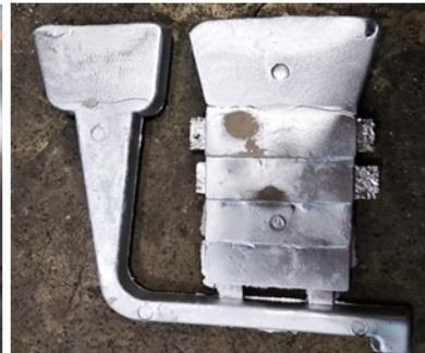
Figure 19: Insertion of foam cores in casting experiments
