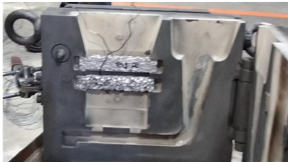
Figure 19: Insertion of foam cores in casting experiments
