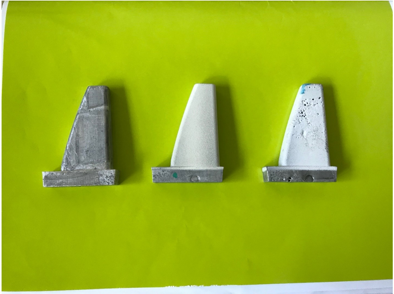
Figure 87: (from left to right) Uncoated foam, Zirconia coated foam and alumina coated foam
