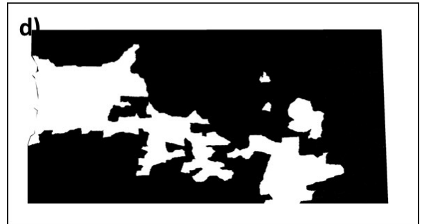
Figure 81: The residual porosity of 3S1 is 36.6%
