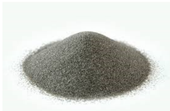
Figure 9: Titanium Hydride \text{TiH}_2 powder[5]
