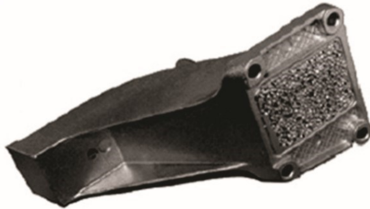
Figure 15: Prototype of a BMW engine mounting bracket[11]
