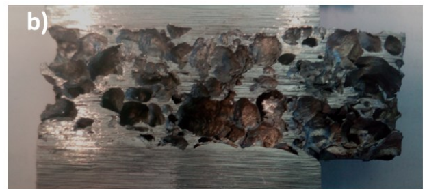
Figure 81: The residual porosity of 3S1 is 36.6%
