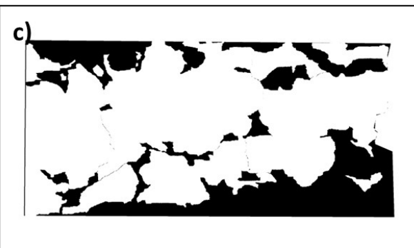
Figure 82: the residual porosity of 4S1 is 69.8%
