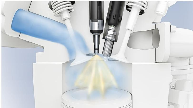
Figure 1.1: Gasoline Direct Injection system example [9]
