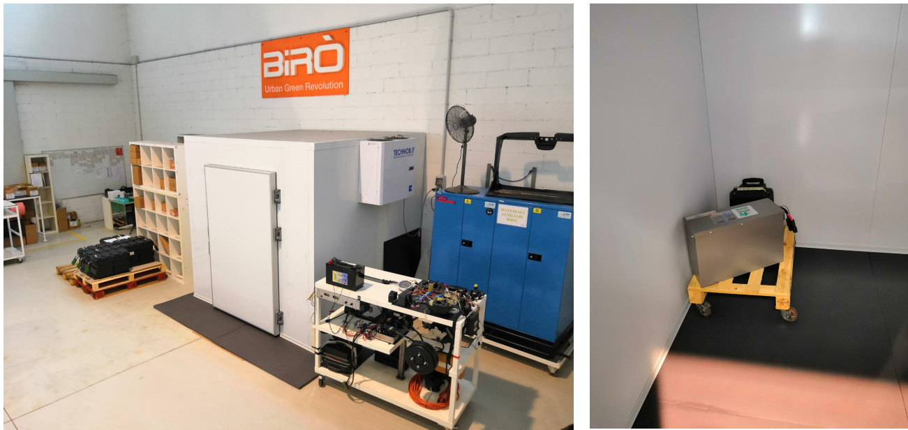
Figure 4.22 Refrigerator used for testing the vehicles and the lithium batteries under temperature levels reaching -20^{\circ}\text{C}
