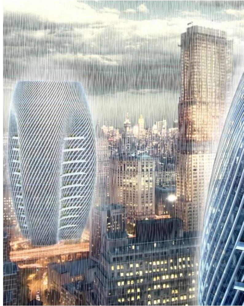
“The Rain Skyscraper is a building whose roof and external shell ,which consists systems of gutters, are aimed at capturing as much rainfall as possible to meet the daily needs of its inhabitants. Under a roof’s surface, there are water reservoirs in the form of a large funnel and reed fields, which serve as a hydro botanic water treatment unit. The unit processes water into usable water that is further transmitted to
