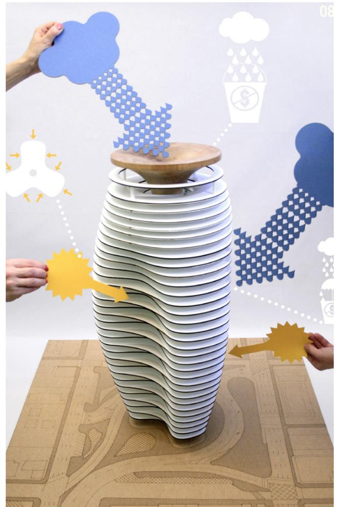
apartments. A network of gutters on the external surfaces of the building is designed to capture rainfall flowing down the building. Such flowing rainfall is transmitted to floors and its surplus is stored in a reservoir under the building. Water captured and processed by the building may be used for flushing toilets, feeding washing machines, watering plants, cleaning floors and other domestic applications.”
