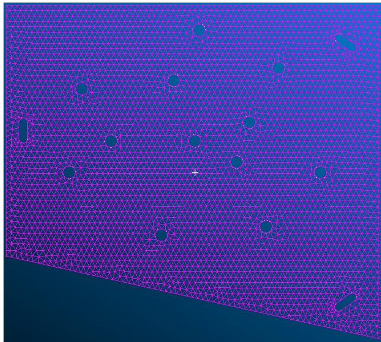
Figure 23- Mesh with about 50000 nodes
