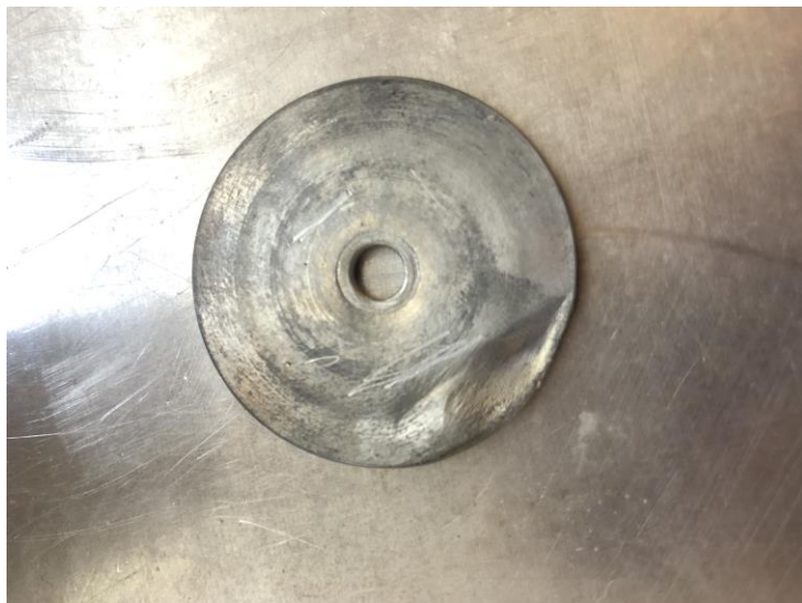
Figure 76-Washer deformation in the upper part
