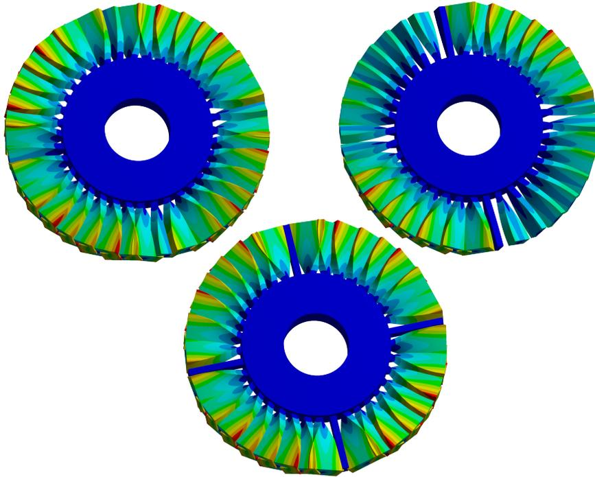
Figura 3.7: Turbine rotor with torsional mode characterized by various nodal diameter but no nodal circumference.
