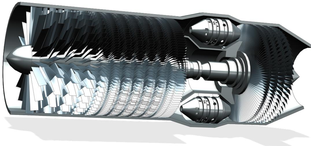
Figura 1.7: A turbojet engine section view.
