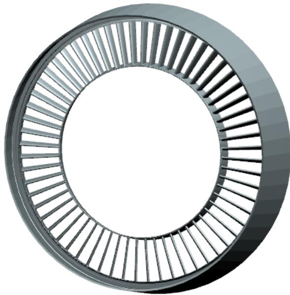
Figura 1.21: Row of turbine nozzle with casing.
