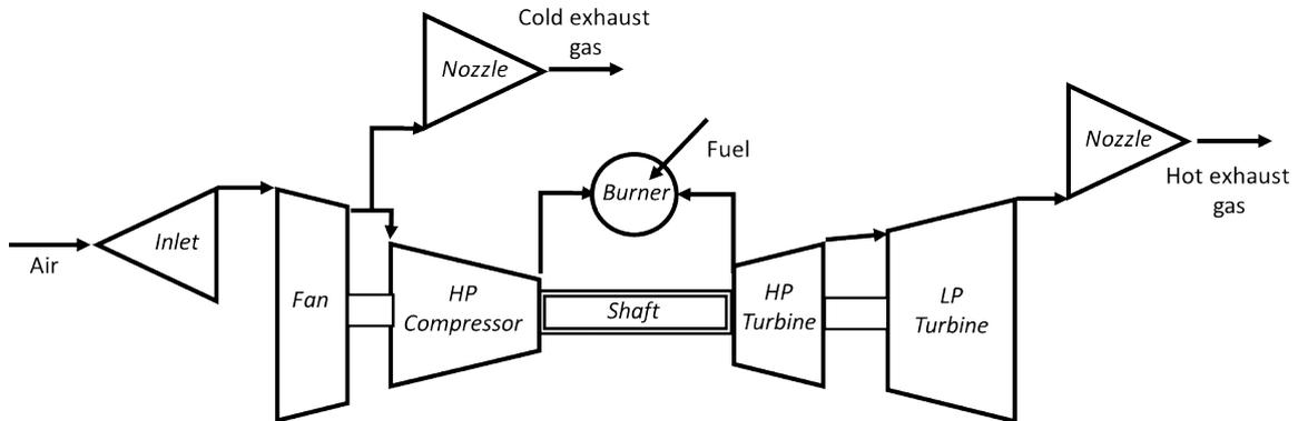
Figura 1.8: Basic scheme of a turbofan engine.
