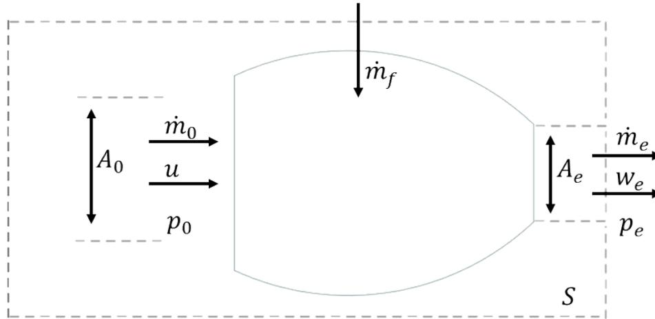
Figura 1.3: Control surface for thrust evaluation.
