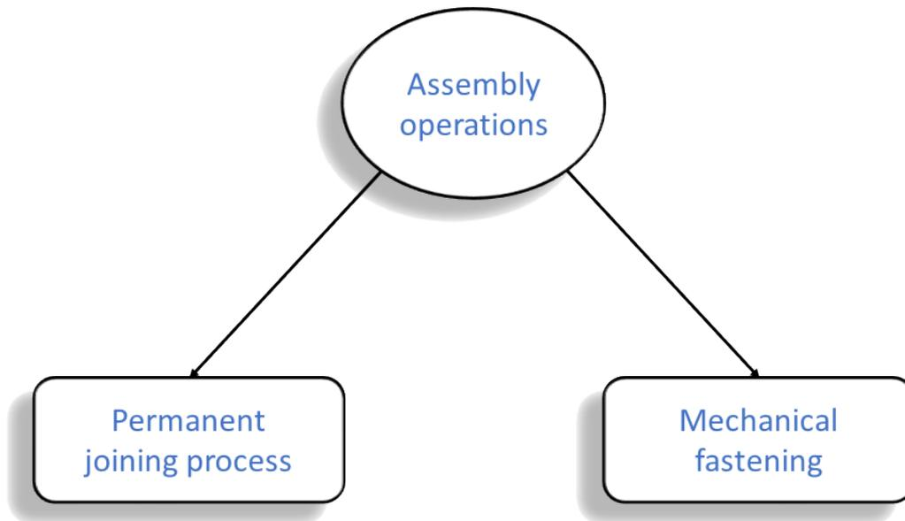
Figura 5.2: Assembly operations scheme.
