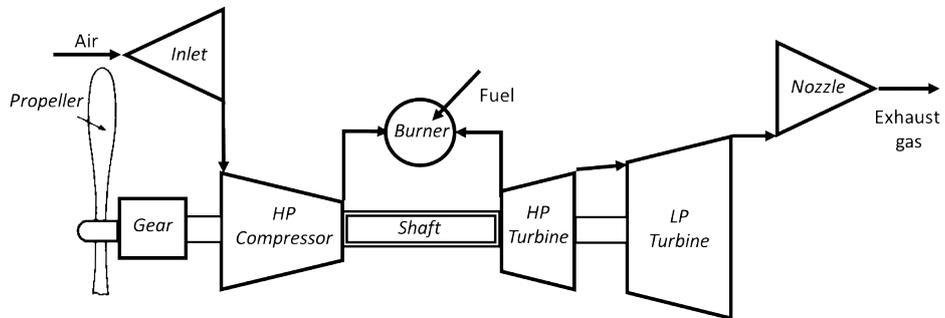
Figura 1.11: Basic scheme of a turboprop engine.
