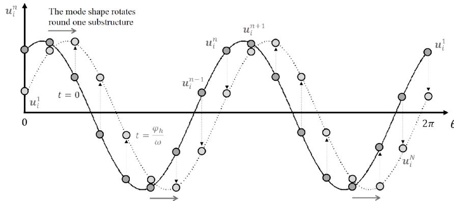
Figure 3.10: Rotating wave mode shapes with moving peaks.[7]
