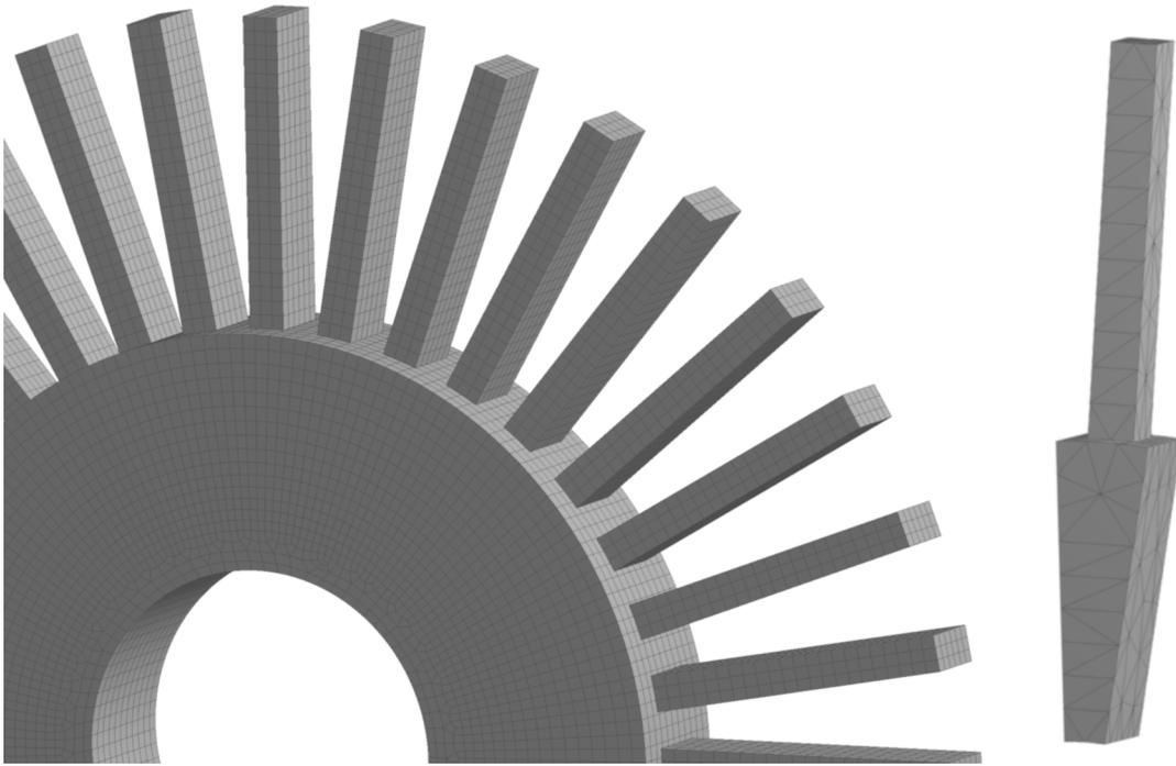
Figura 3.16: Meshed model of a dummy turbine rotor.
