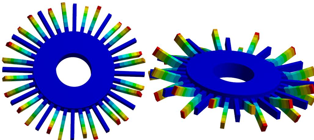
Figura 3.6: Turbine rotor with bending mode shape characterized by six nodal diameter and no nodal circumference.
