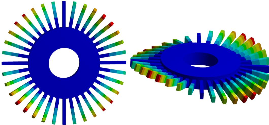
Figura 3.5: Turbine rotor with bending mode shape characterized by two nodal diameter and no nodal circumference.
