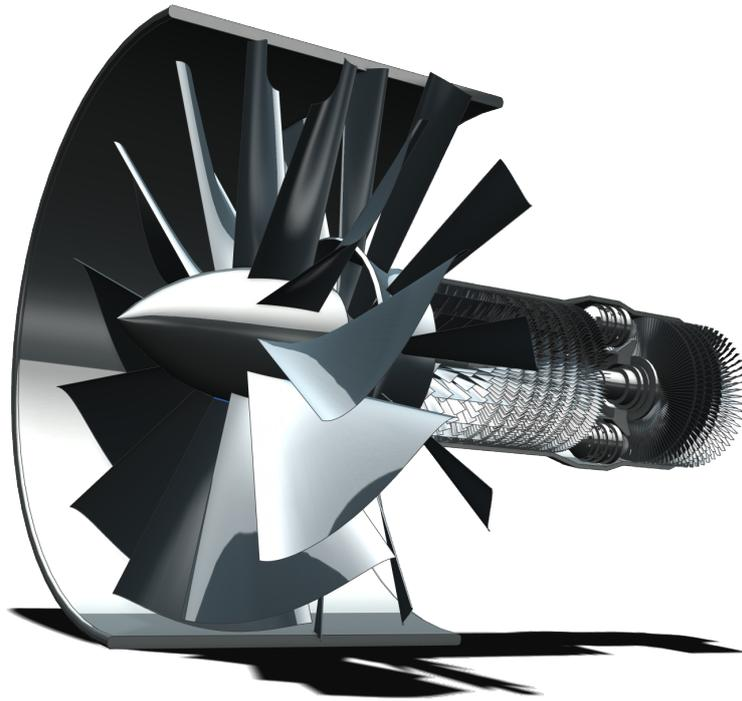
Figura 1.10: A turbofan engine section view.
