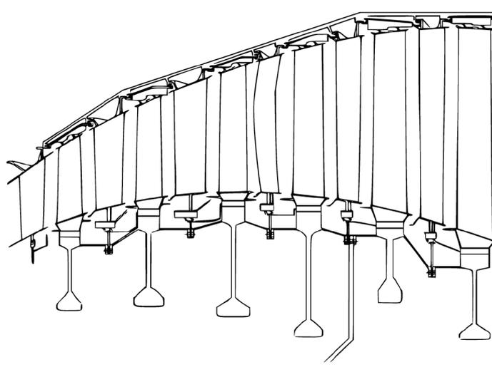
Figura 1.15: A low pressure turbine section.
