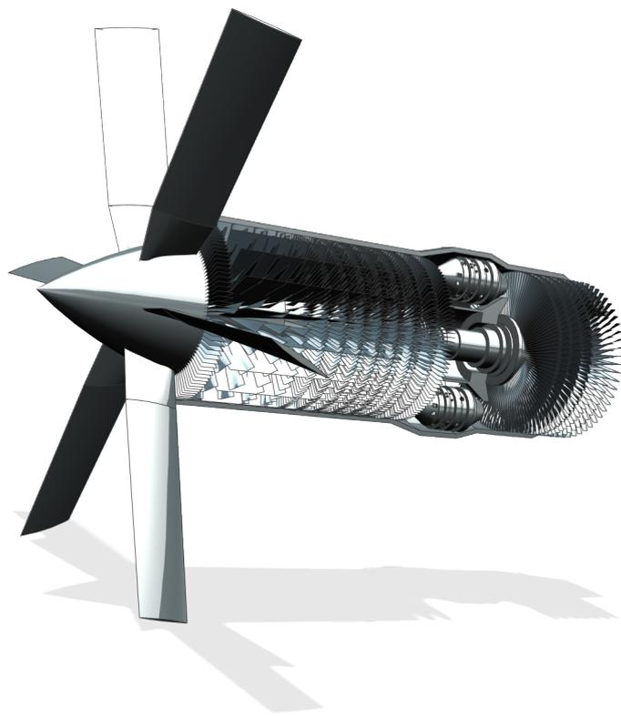
Figura 1.13: A turboprop engine section view.
