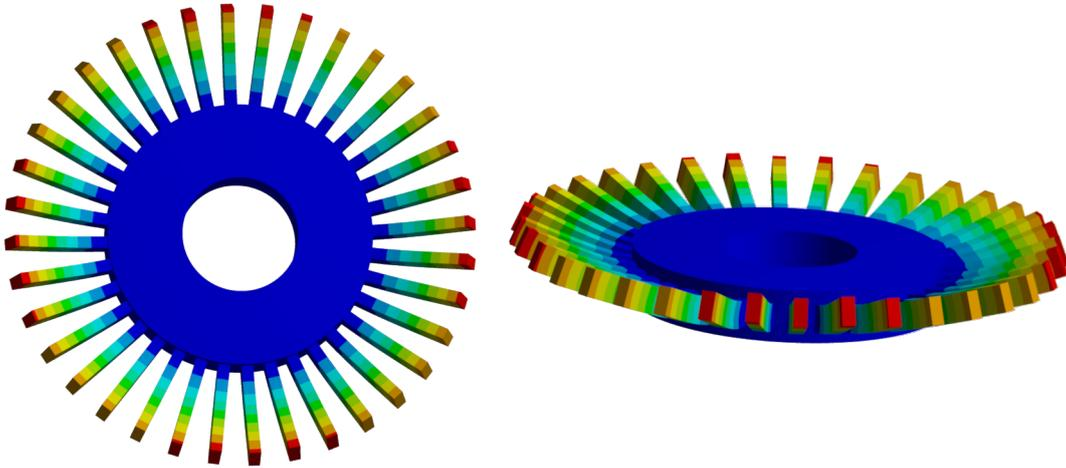
Figura 3.3: Turbine rotor with bending mode shape characterized by no nodal diameter and no nodal circumference.
