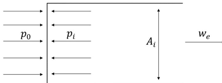
Figura 1.1: Simplified model of a jet propulsion engine.
