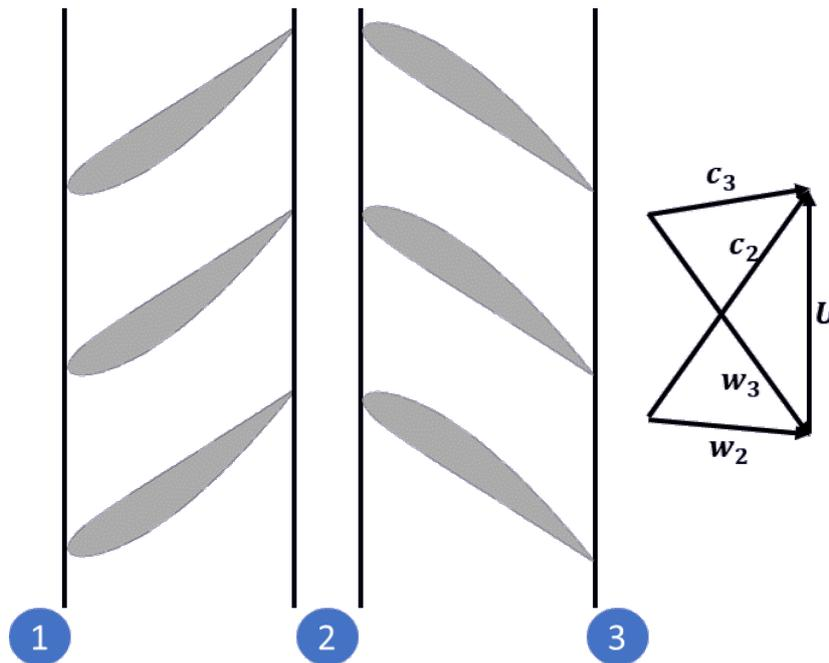
Figure 1.16: Typical turbine stage section and velocity diagram.
