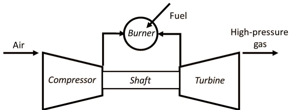
Figura 1.4: Basic gas generator scheme.
