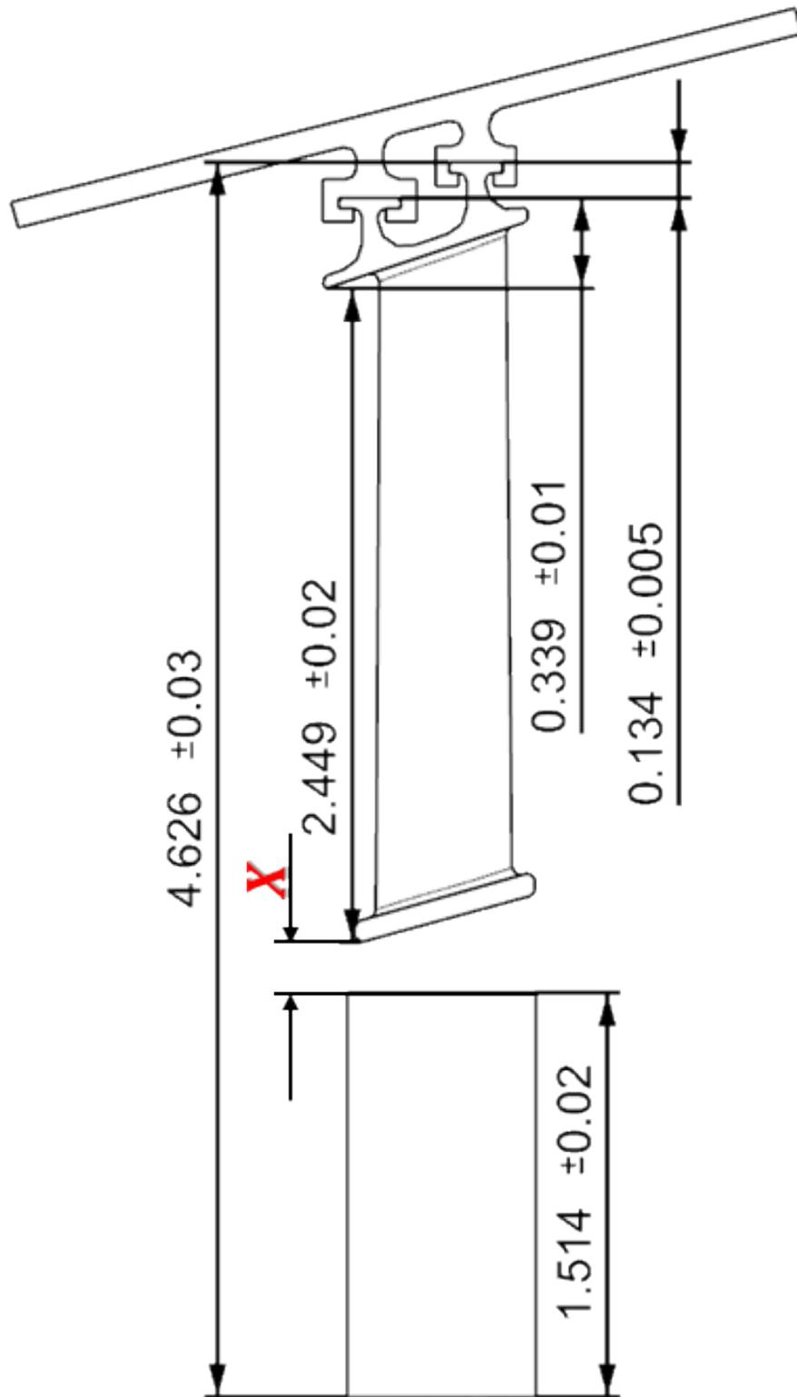
Figura 7.1: Example for tolerance stackup analysis.
