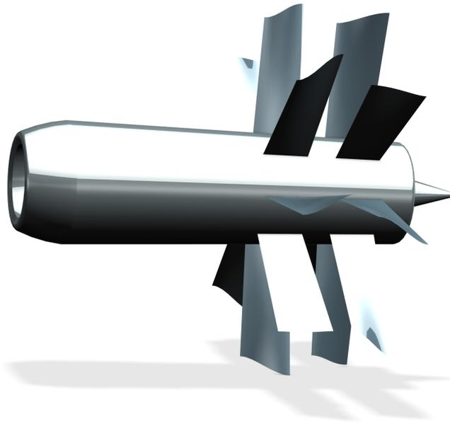
Figura 2.4: Open Rotor concept model.
