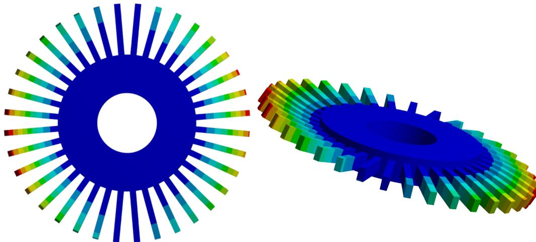
Figura 3.4: Turbine rotor with bending mode shape characterized by one nodal diameter and no nodal circumference.
