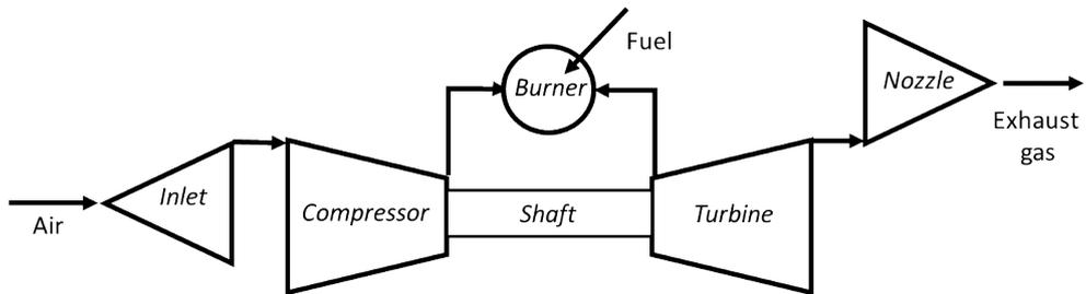
Figura 1.5: Basic scheme of a turbojet engine.
