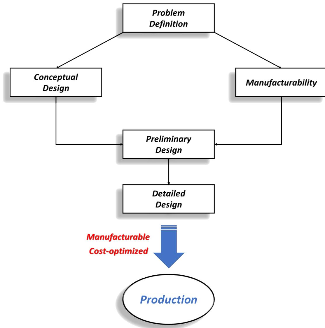
Figura 6.4: DFM-based design process.
