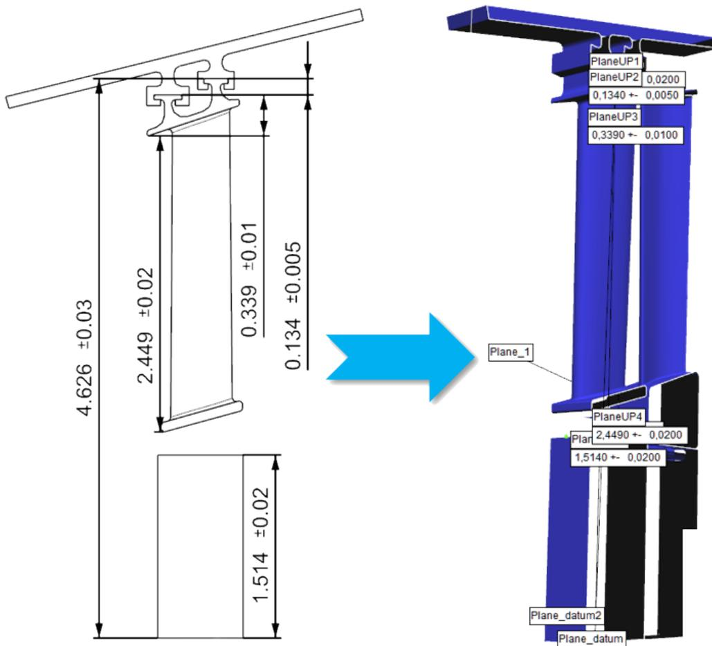
Figure 7.4: Modeling and PMI definition of the test case.
