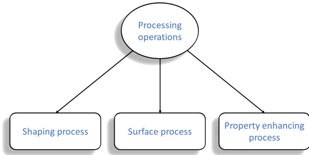
Figura 5.1: Processing operations scheme.
