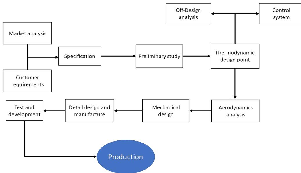
Figure 1.14: The design process flow chart.
