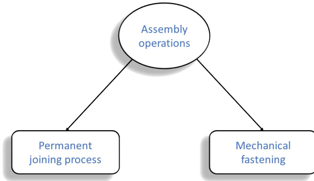
Figura 5.2: Assembly operations scheme.
