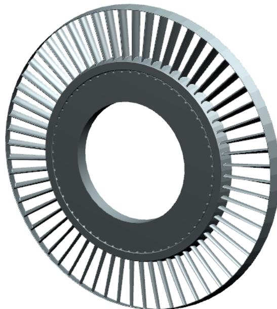
Figura 1.20: Row of turbine bladed disk.
