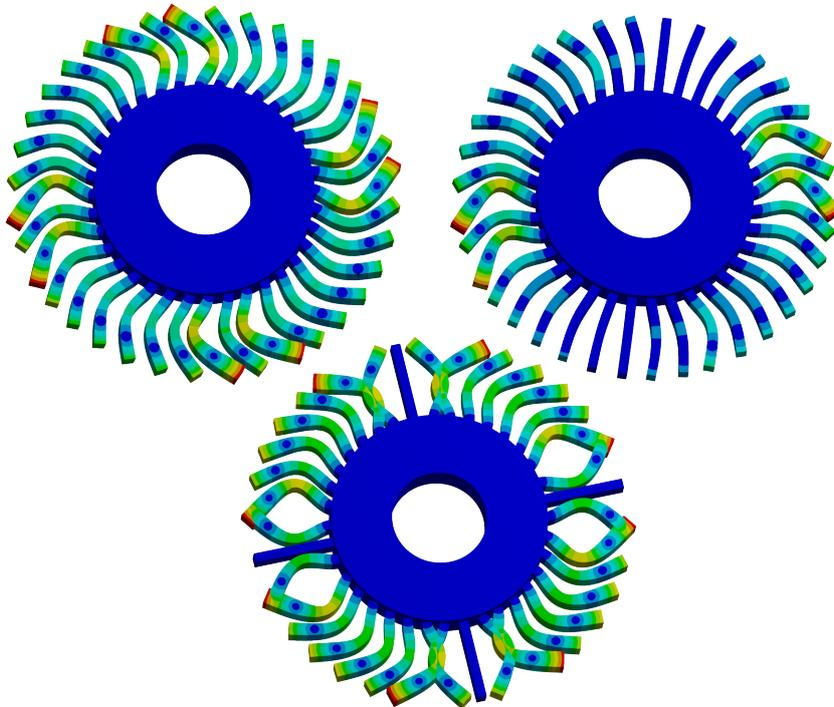
Figura 3.8: Turbine rotor with bending mode characterized by one nodal circumference but no nodal diameter.
