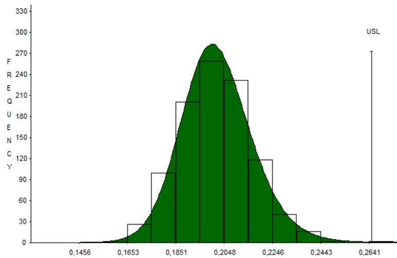
Figura 7.6: Results comparison with worst case tolerance analysis.
