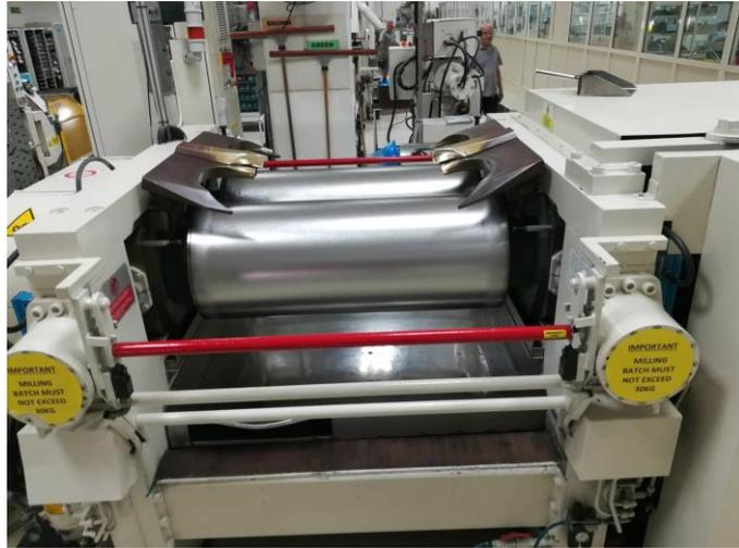
*Figura 12 – Open Rubber Milling machine*
