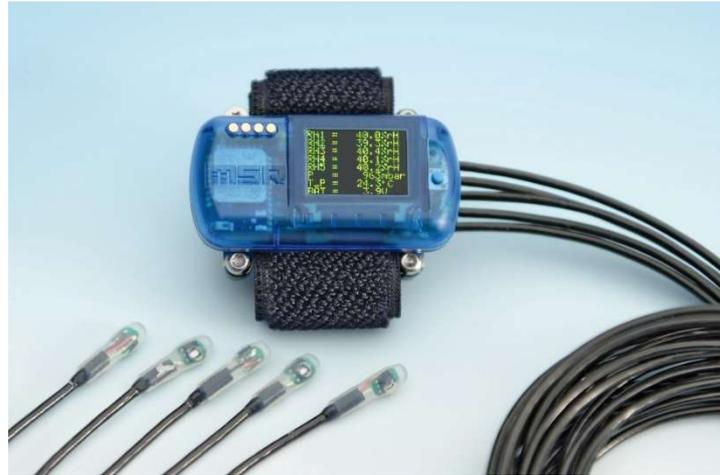
**Fig. 5. 8:** data logger MSR147WD
