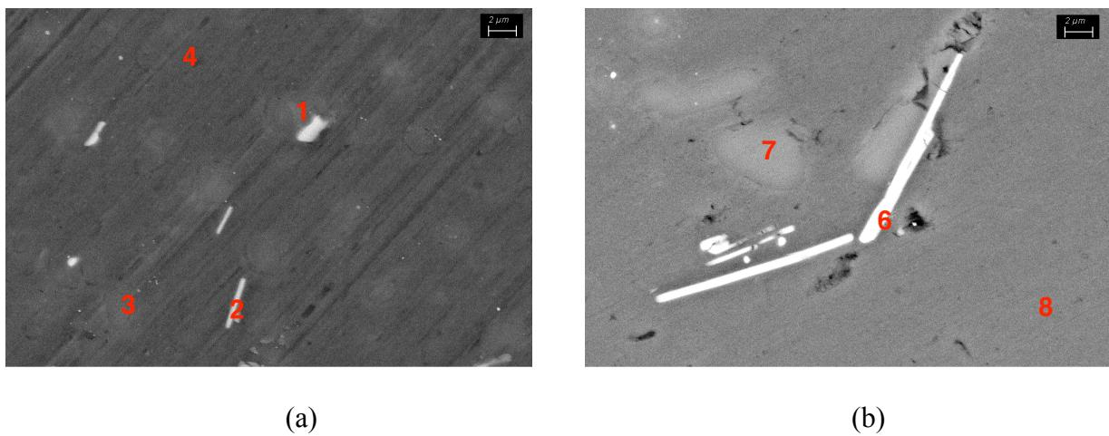
**Fig. 5.7** EDS analysis on the samples, (a) AM sample, Fe-rich precipitates, Al matrix and Si grains at the Al grain boundaries, (b) Cast sample, Fe-rich precipitates, Al matrix and Si grains segregation at the grain boundaries of rather large Al crystals.
