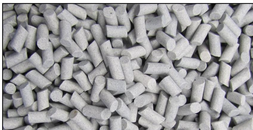
**Fig 3.5** Abrasive used in tumbling
