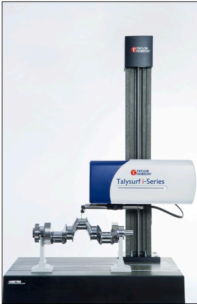
**Fig. 4.18** TALYSURF PLUS profilometer
