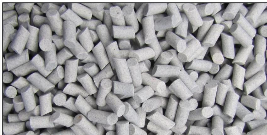
**Fig 3.5** Abrasive used in tumbling
