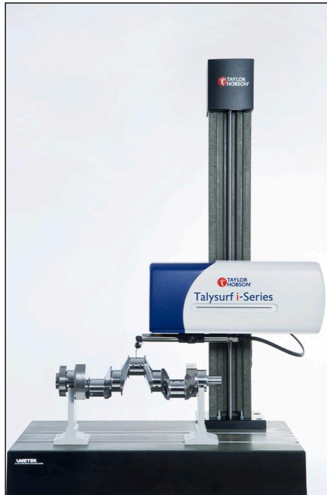
**Fig. 4.18** TALYSURF PLUS profilometer
