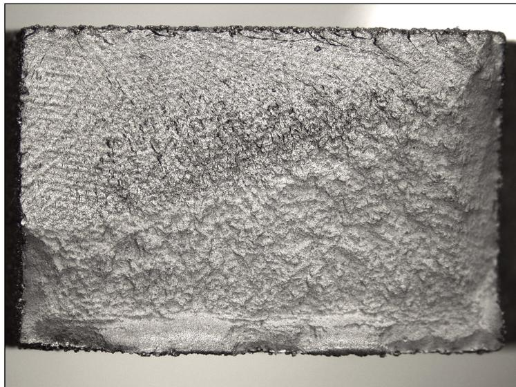
**Fig 1.2** A fatigue fracture on a AM specimen
