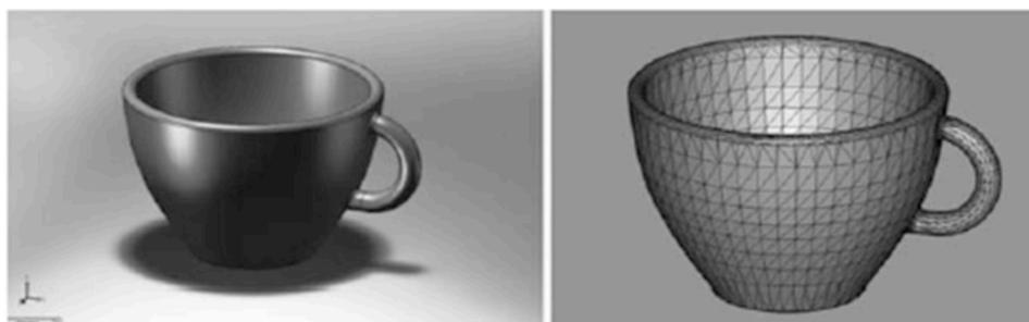
**Fig 2.1** A CAD model on the left converted into STL format on the right. [2]
