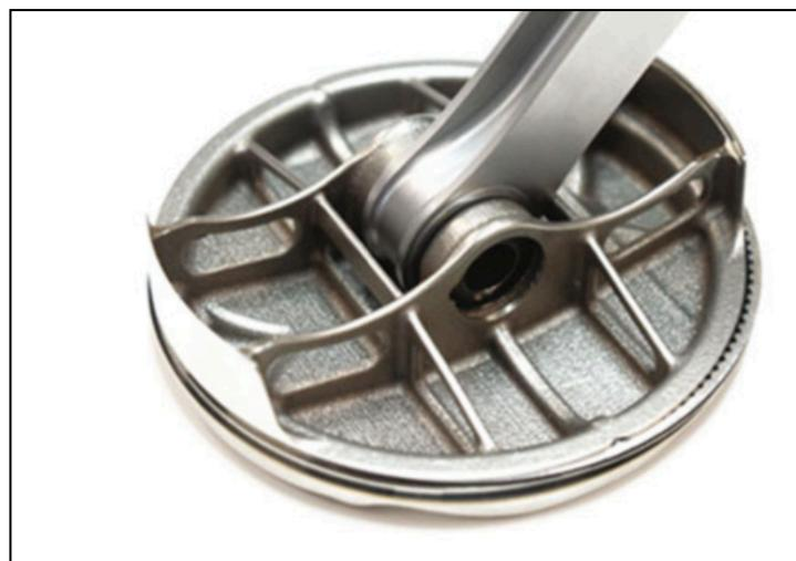
**Fig 2.8** Piston made by AM[5].
