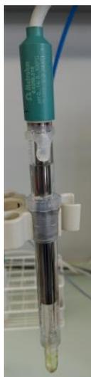
**Figure 4.5: Metrohm combined pH electrode with integrated Pt1000 temperature sensor and fixed cable (1.2 m, diameter banana plug 2 mm). Order number 6.0258.010.**
