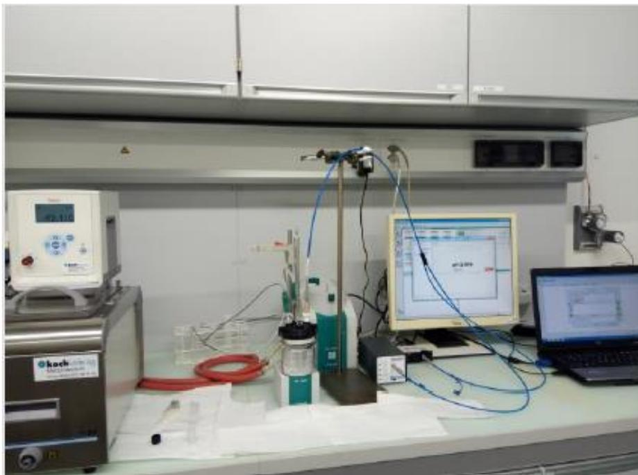
Figure 4.1: Setup for synthesis and characterization in situ of colloidal gold
