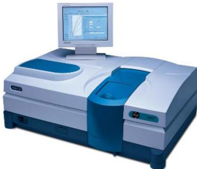
Figure 4.9: Varian Cary 4000 UV-vis-NIR Spectrophotometer.<sup>45</sup>
