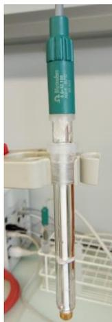
**Figure 4.4: Metrohm combined gold ring electrode with a ceramic pin diaphragm order number 6.0452.100.**
