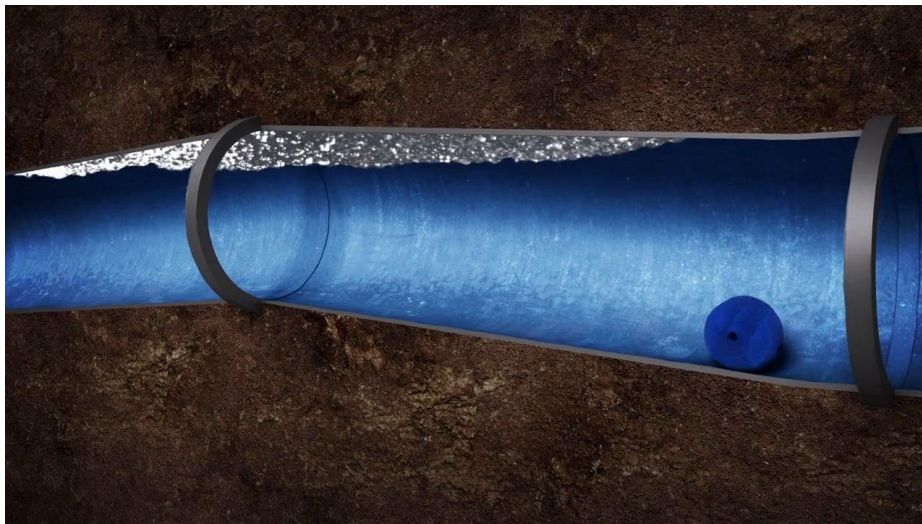
Figure 15. representation of a SmartBall operating inside a water pipeline
