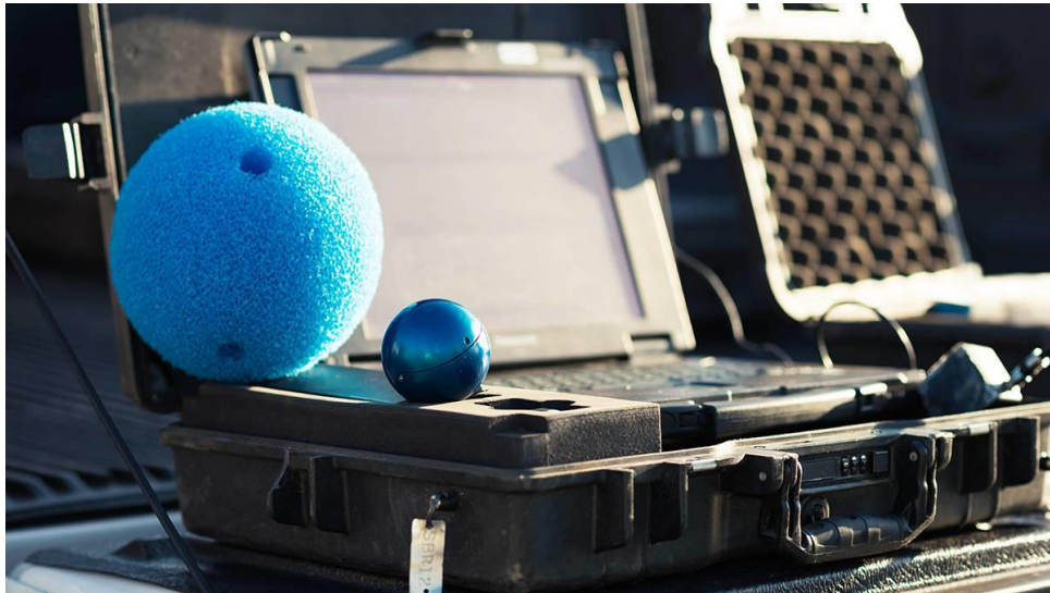
Figure 16. SmartBall outer rubber foam sphere (left) and inner aluminium sphere (right)
