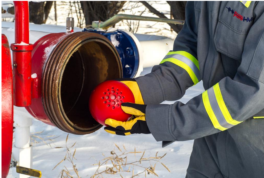
Figure 26. Insertion of SmartBall® inside an oil pipeline
