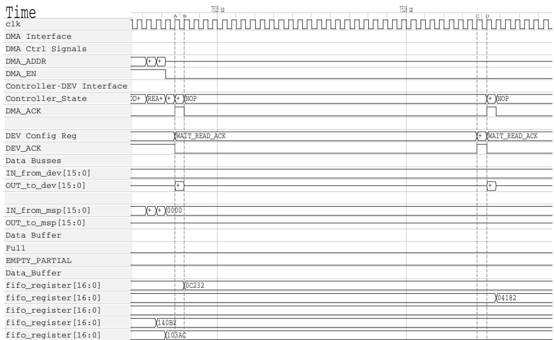
Figure 6.12: Sending data to a device directly connected to the controller. The communication protocol between the two implies a 2-phase handshake: the device requests data by raising its acknowledge signal (marker A); the controller drives the output data and flags the sending through its own acknowledge signal (marker B).
