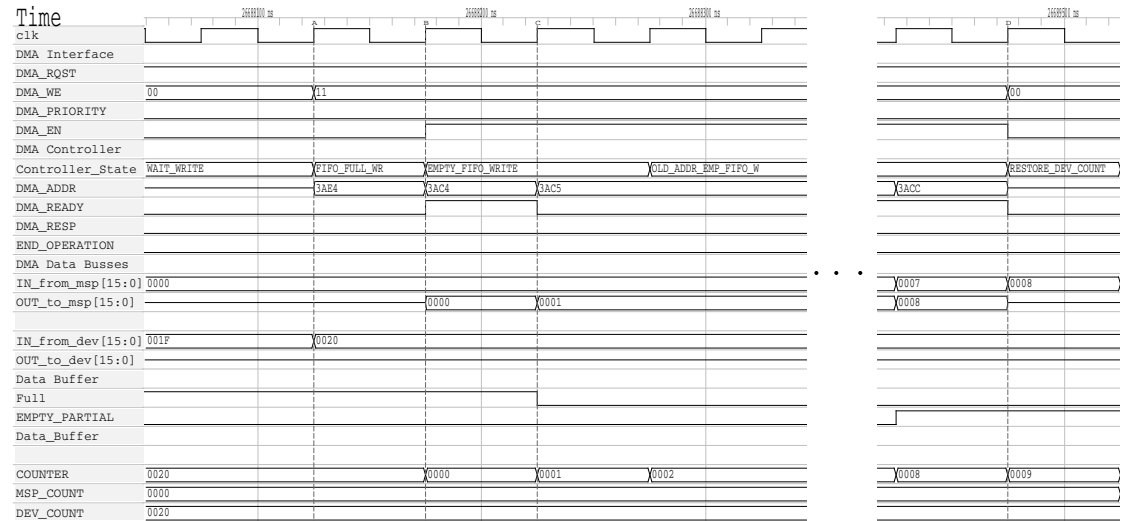
Figure 6.17: Emptying the controller data buffer by outputting data to system memory.
