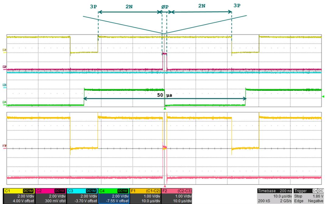
Fig. 2.31 SVM SECTOR 5 - C1: U High, C2: V High, C3: W High, C4: SPI int, F1: differential mode Uh-Vh, F2: differential mode Vh-Wh.
