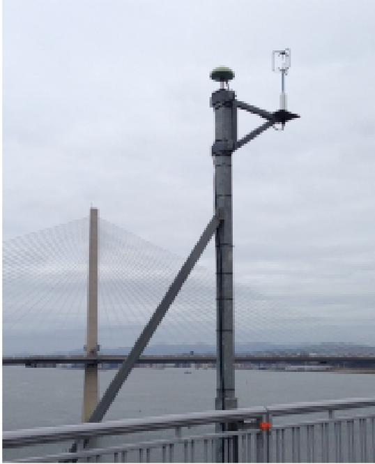
*Figure 4.12: 3D sonic anemometer at midspan*
