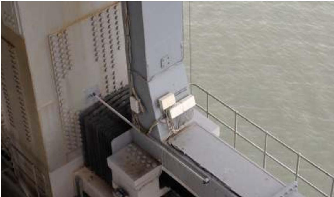
*Figure 4.9: Displacement transducer at the bottom of the end post at NEMS*
