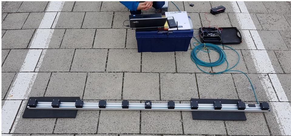
Figure 2.5: Complete MSAS: The sensor array is connected through a single cable to the array controller, which is connected to the GPS antenna and to a 12 V battery that powers the whole system. The array controller is USB connected to a laptop for data storage and analysis.
