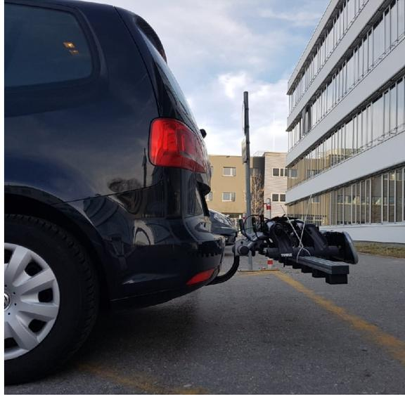
Figure 4.1: Experiment setup: The MSAS is placed behind the road vehicle, as far as possible from the electro-magnetic disturbances generated by the car.
