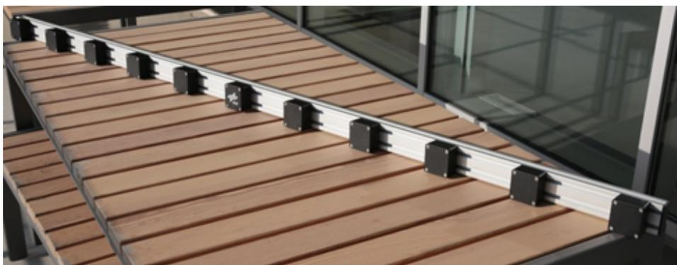
Figure 2.3: MSAS in its operational setup: 11 boxed sensor elements are fixed on the aluminum pole.
