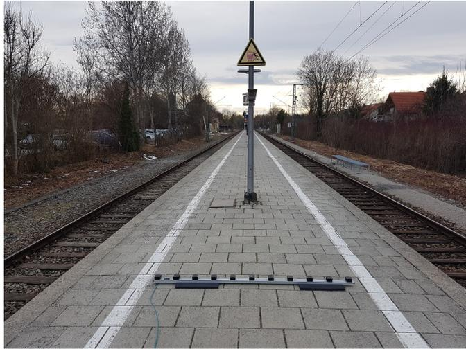
Figure 5.1: Experiment setup: The MSAS is placed on the platform, perpendicular to the train direction of motion and at the same distance from left and right tracks. Sensor element 1 is on the left side of the picture, sensor element 11 is on the right side.
