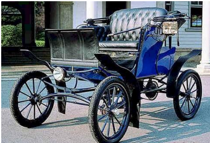
Figure 1: 1903 Baker Electric – There is no steering wheel. It was steered with a tiller, visible above in front of the driver's seat on the left of the vehicle [1].
