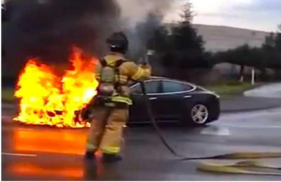
Figure 16: A Tesla model S car caught fire due to lithium-ion battery explosion [29].
