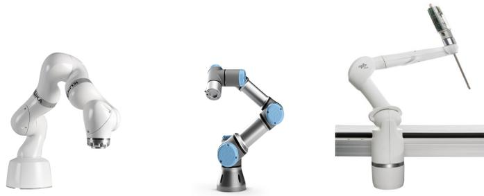
FIGURE 2.26: From left to the right: KUKA lbr Med 7 R 800 from KUKA (Germany), UR3 from Universal Robots (Denmark) and DLR MIRO from DLR (Germany) [63][64][58].
