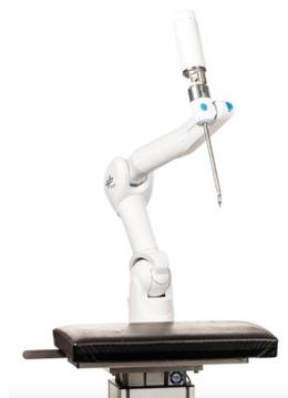
FIGURE 2.22: DLR Miro surgical robot arm [58].
