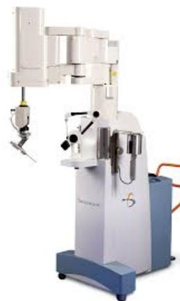
FIGURE 2.13: ROBODOC surgical robotic system [39].
