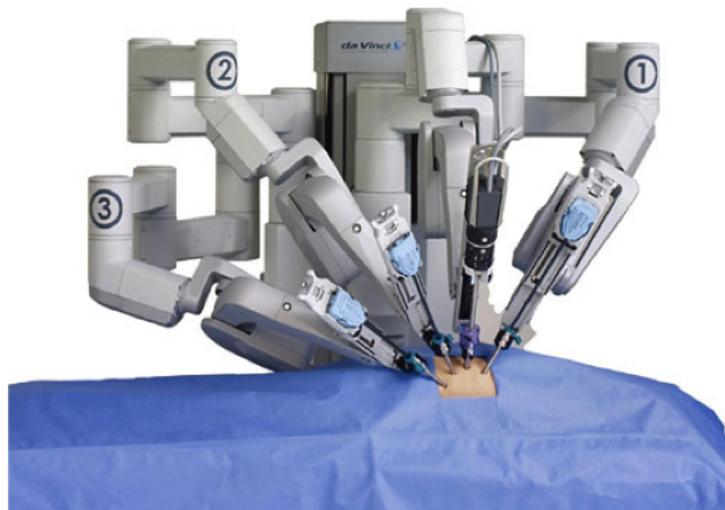
FIGURE 1.2: Da Vinci's surgical robotic system assisting in surgery [4].
