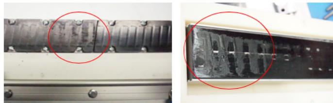
FIGURE 3.9: Stacking zone of the coil part and magnets.
