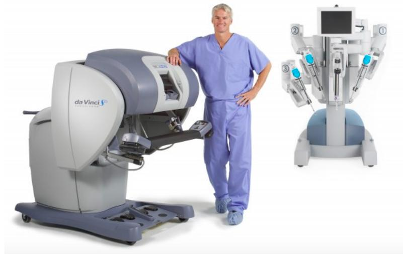
FIGURE 2.16: Da Vinci's S version with additional fourth arm [46].
