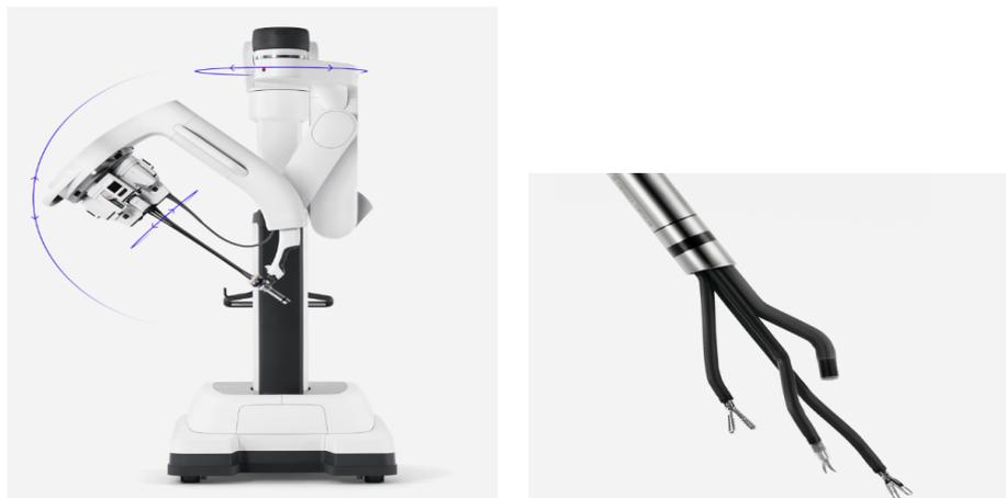
FIGURE 2.17: Da Vinci's SP version and the single multi-wristed arm [51].
