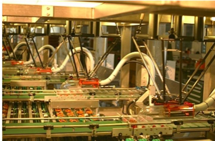
FIGURE 2.6: Demaurex’s Line-Placer installation for the packaging of pretzels in an industrial bakery [26].
