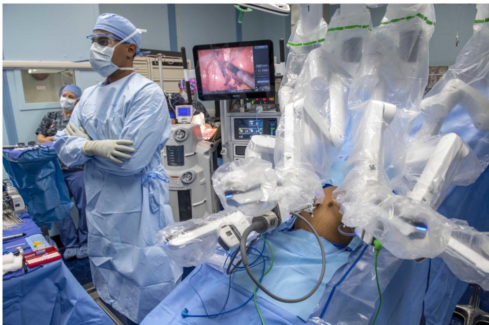
FIGURE 2.31: Surgical robotic system covered during surgery[69].
