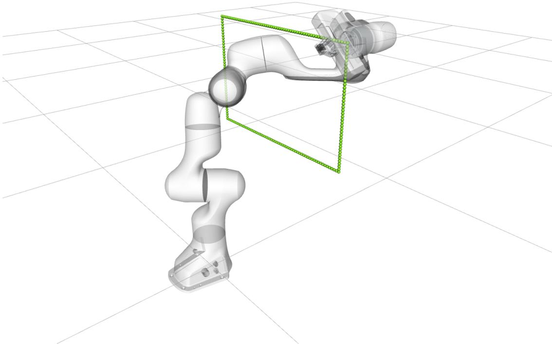
Figure 2.3: Panda manipulator TCP proceeding through trajectory waypoints.
