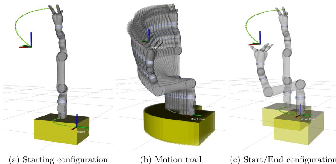
Figure 5.3: Base-arm kinematics plugin applied to a mobile manipulator.
