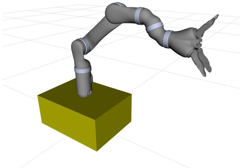
Figure 5.2: Model of mobile manipulator with Kinova Mico as robotic arm.
