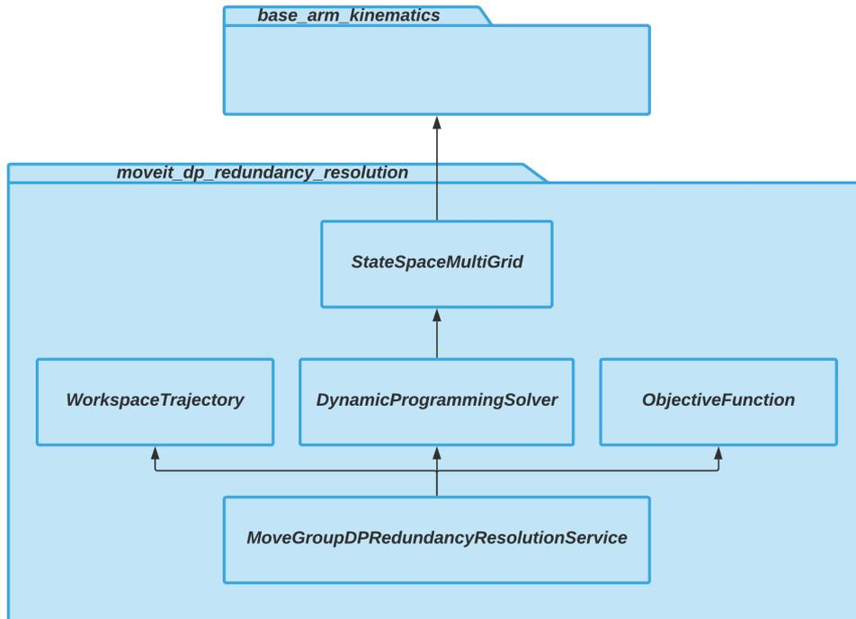
Figure 6.2: UML class diagram depicting the design structure of the service.
