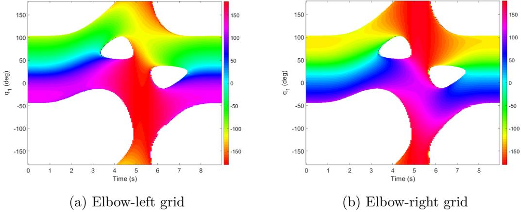
Figure 3.2: Colormaps of homogeneous grids indicating the value of joint  $q_2$ .
