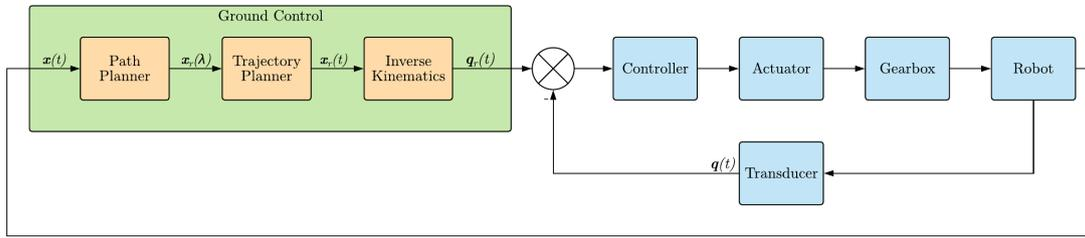
Figure 2.4: Scheme of a closed-loop control system with trajectory planner.
