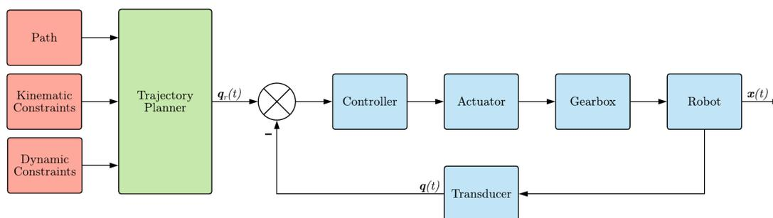
Figure 2.2: Scheme of a trajectory planner followed by a control system.
