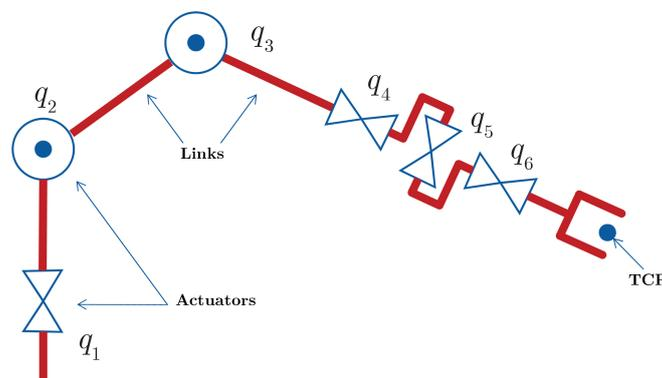
Figure 3.1: Kinematics chain of a 6-DOF manipulator.
