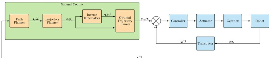
Figure 4.1: Scheme of a closed-loop control system with optimal trajectory planner.
