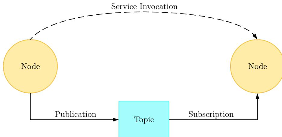
Figure 4.2: Two nodes communicating over a topic during a service invocation.
