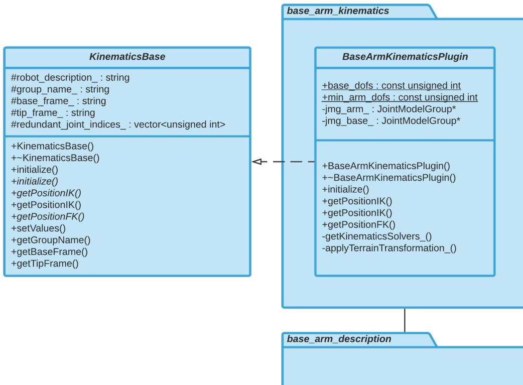
Figure 6.1: UML class diagram depicting the design structure of the plugin.
