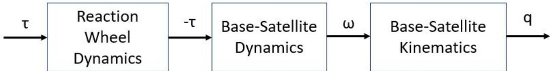
Figure 3.6: Base-satellite model block diagram
