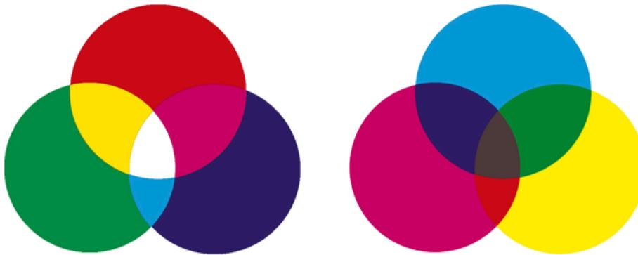
FIGURA 13\_SINTESI ADDITIVA (SINISTRA) E SINTESI SOTTRATTIVA (DESTRA)
