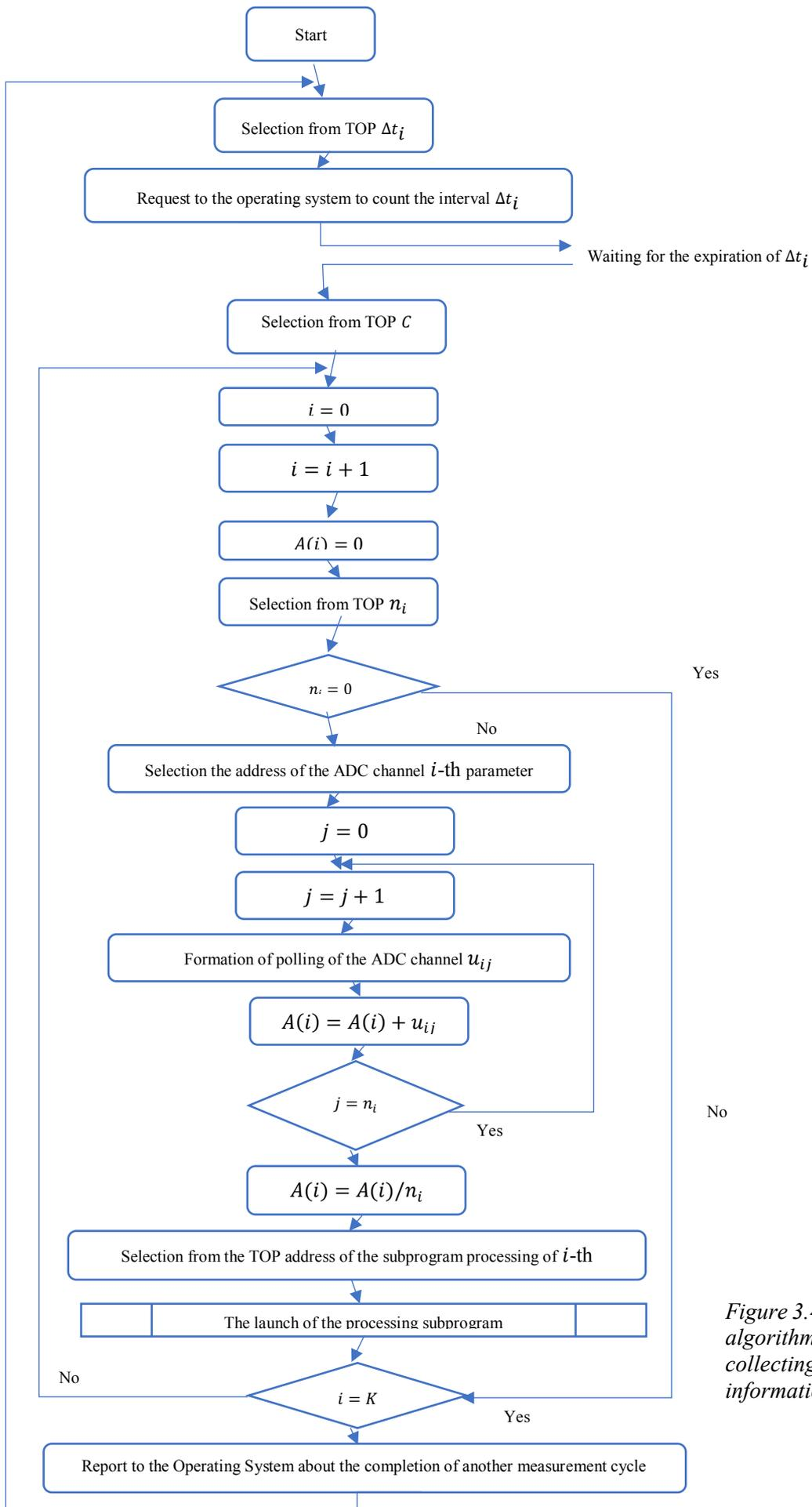
Figure 3.4 The block diagram of the algorithm of the system for collecting and preprocessing information
