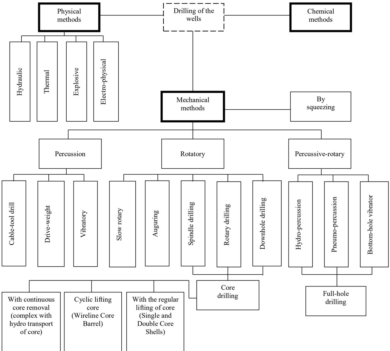
Table 1.1 Classification of mechanical methods of drilling wells
