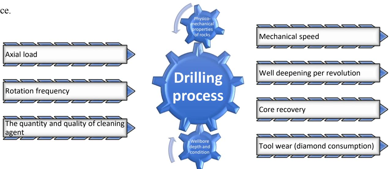
Figure 2.1 The structure of the drilling process model
