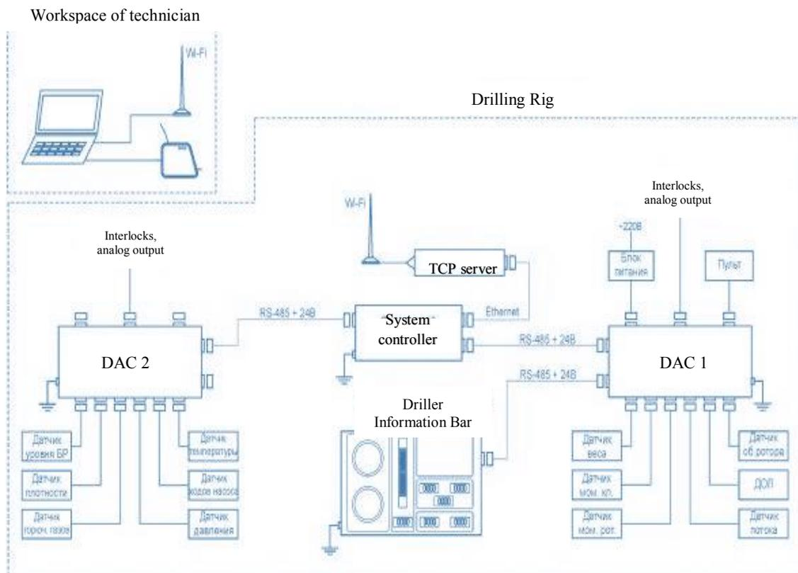
Figure 2.3 Block diagram of the system of technological control of drilling parameters [19]
