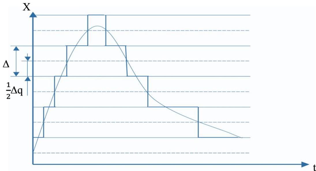
Thus, as a result of quantization of function  $\lambda(t)$ , produced by a certain rule, it is possible to select a series of its discrete values. Actually, with the selection of the points the quantization process ends.
