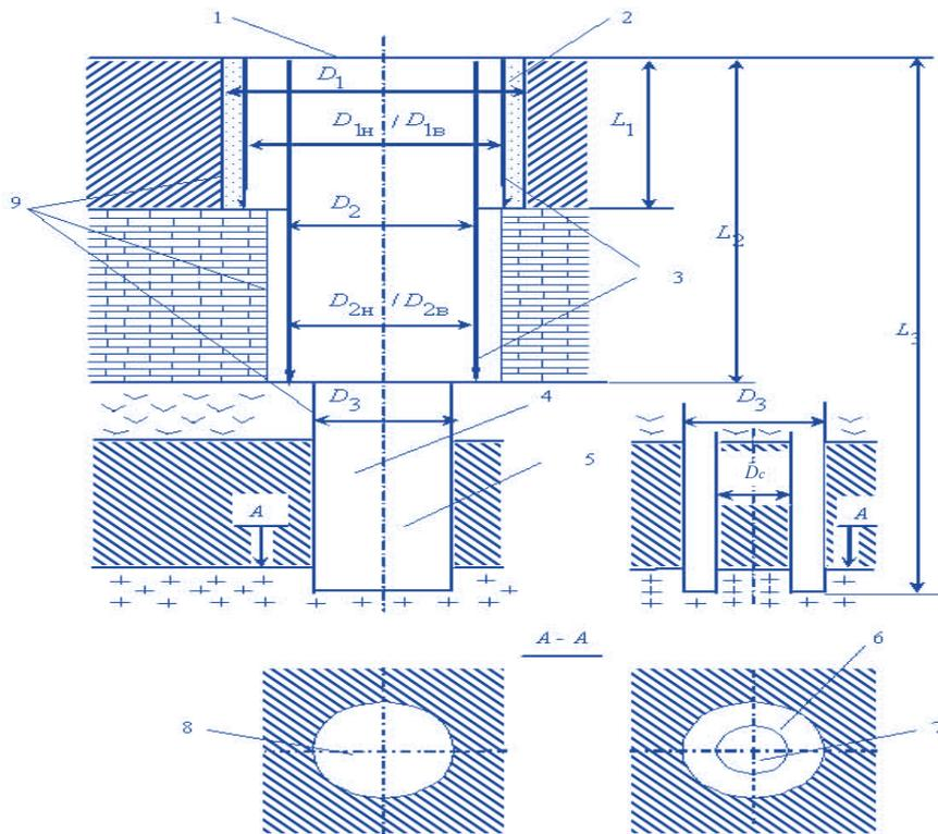
Figure 1.1 Elements of the borehole: 1 - wellhead; 2 - wellbore, cased tubes; 3 - casing strings; 4 - well axis; 5 - wellbore, not cased; 6 - the circular face; 7 - core; 8 - full hole; 9 - well walls;  $D_1$ ,  $D_2$ ,  $D_3$  - borehole diameters in different intervals;  $D_{1i}$ ,  $D_{1o}$ ,  $D_{2i}$ ,  $D_{2o}$  are the casing diameters, respectively, external, internal;  $D_c$  - core diameter;  $L_1$ ,  $L_2$  - the depth of the intervals of the well, cased;  $L_3$  - well depth. [9]
