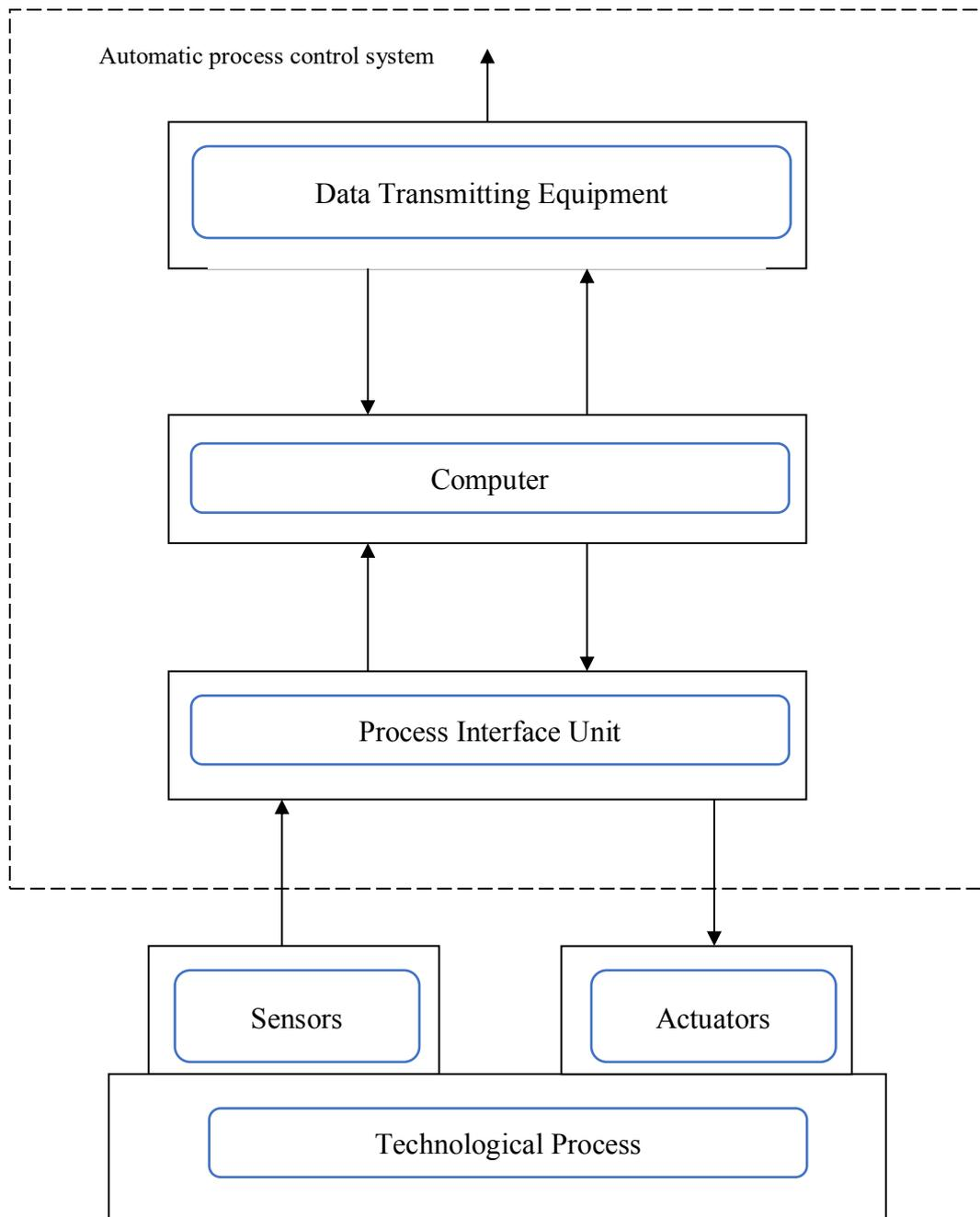
*Figure 4.1 The typical structure of the automated process control system based on the control computer.*
