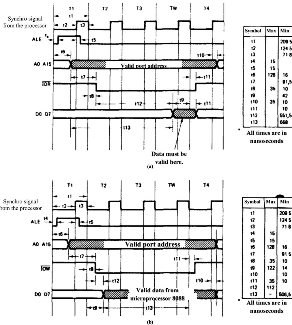
Figure 4.2 Timing diagrams of the input-output port. Time distribution of the bus read cycle for the input port (a) Time distribution of the bus write cycle for the output port (b). [20]
