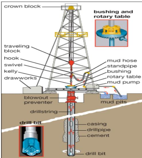
Figure 1.5 Rotary drilling rig [22]
