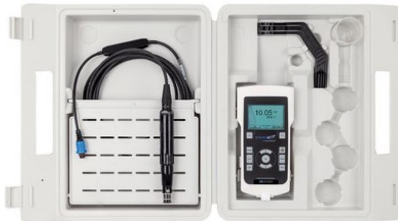
*Figure 3-3. VWR pHenomenal® OX 4100 dissolved oxygen and pH meter.*
