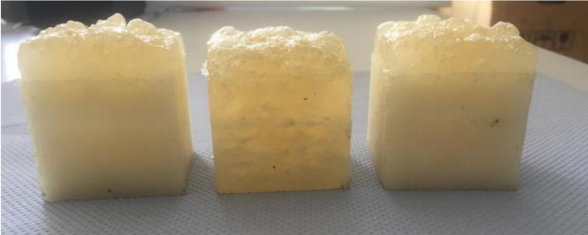
**Figure 17: Cured resin slurry contaminated with 5% spacer/mud**
