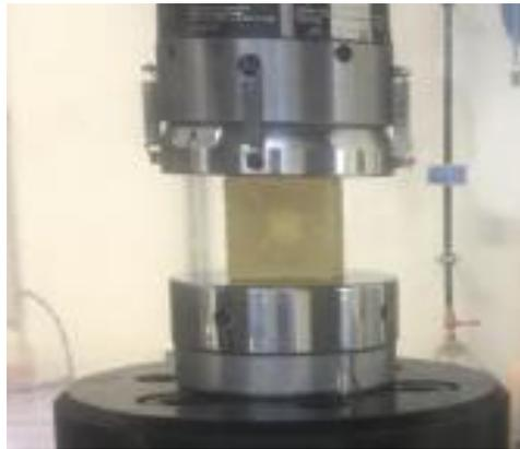
**Figure 16: Hydraulic press for compressive strength measurement**
