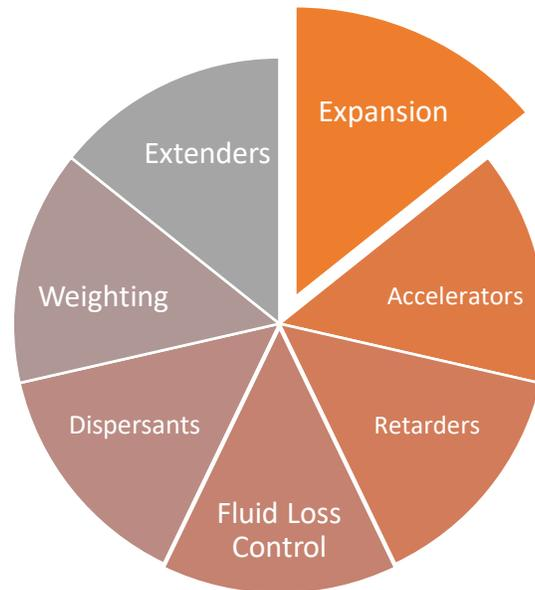
**Figure 6: Classification of additives for well cementing**
