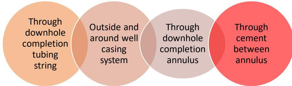
**Figure 4: Ways of losing well integrity**
