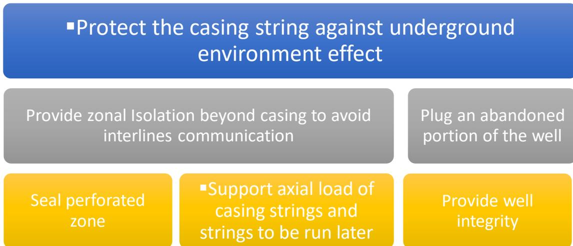
**Figure 7: Purpose of cementing jobs**
