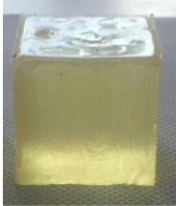
**Figure 15: Cured resin system for compressive strength measurement**
