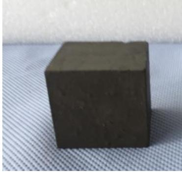
**Figure 11: Cured conventional cement for compressive strength measurement**
