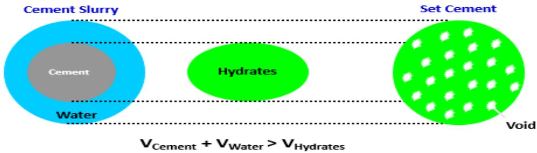
**Figure 8: Schematic cement hydration process (Schlumberger, 2014)<sup>2</sup>**
