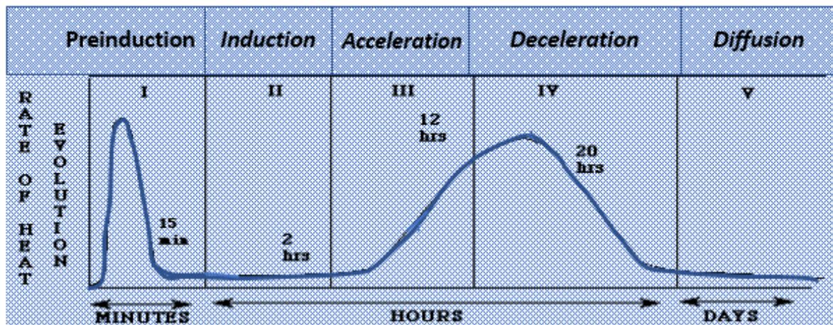
**Figure 5: Hydration stages of cement**
