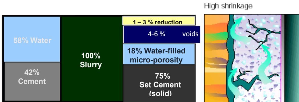
**Figure 9: Representation of volume reduction of concrete (Schlumberger 2014)<sup>2</sup>**
