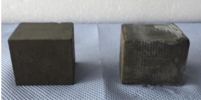
**Figure 14: Cured MRBC system for compressive strength measurement**
