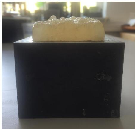
**Figure 18: Cured resin slurry contaminated with 5% spacer/mud**
