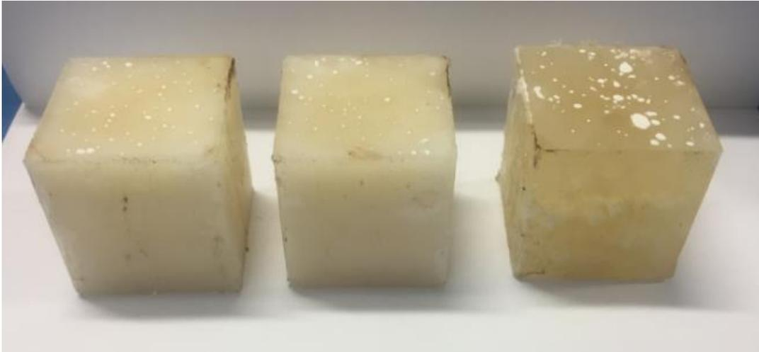
**Figure 20: Cured resin slurry contaminated with 5% diesel**
