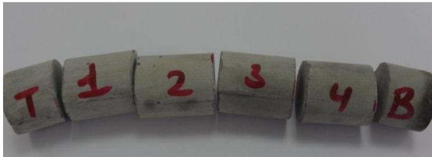
**Figure 12: Cured conventional cement sample for sedimentation measurement**
