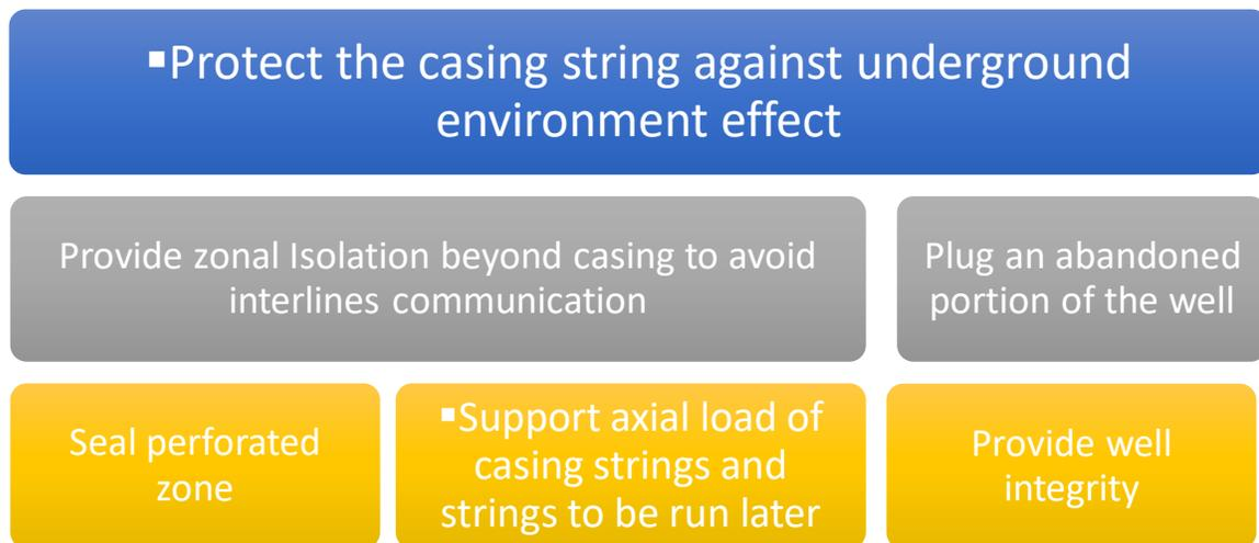
**Figure 7: Purpose of cementing jobs**
