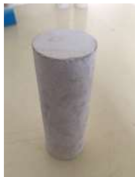
Figure 1 Core sample with 30mm diameter and 100mm height
