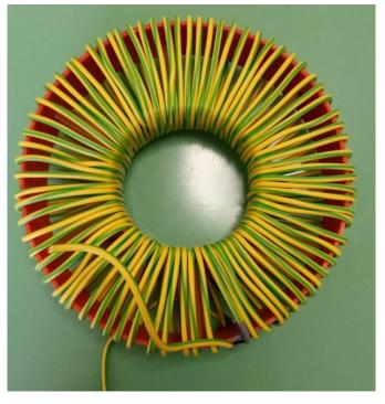
Figure 5.1: Air core toroid.
