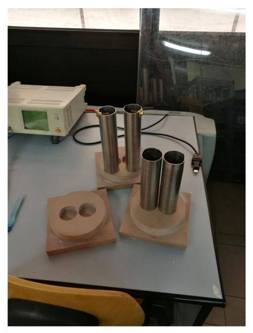
Figure 3.12: Real prototype with electodes of 200 mm and distance d = 2 mm
