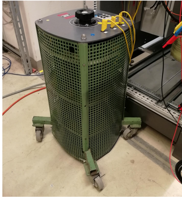
Figure 6.1: The autotransformer, thanks to its ability to manually tune the output voltage, tests were conducted despite the defected relay and three-phase connector.
