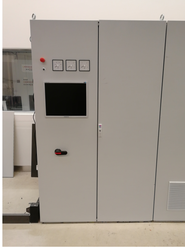
Figure 5.17: The close cabinet: three analog sensors are mounted, a desktop through which the DSP can be debugged and Labview user interface executed.
