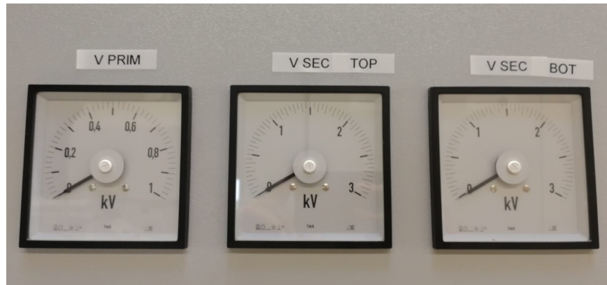
Figure 5.19: The analog meters. On the first it is possible to read the low DC-link voltage, on the other ones the two voltages on the NPC side.
