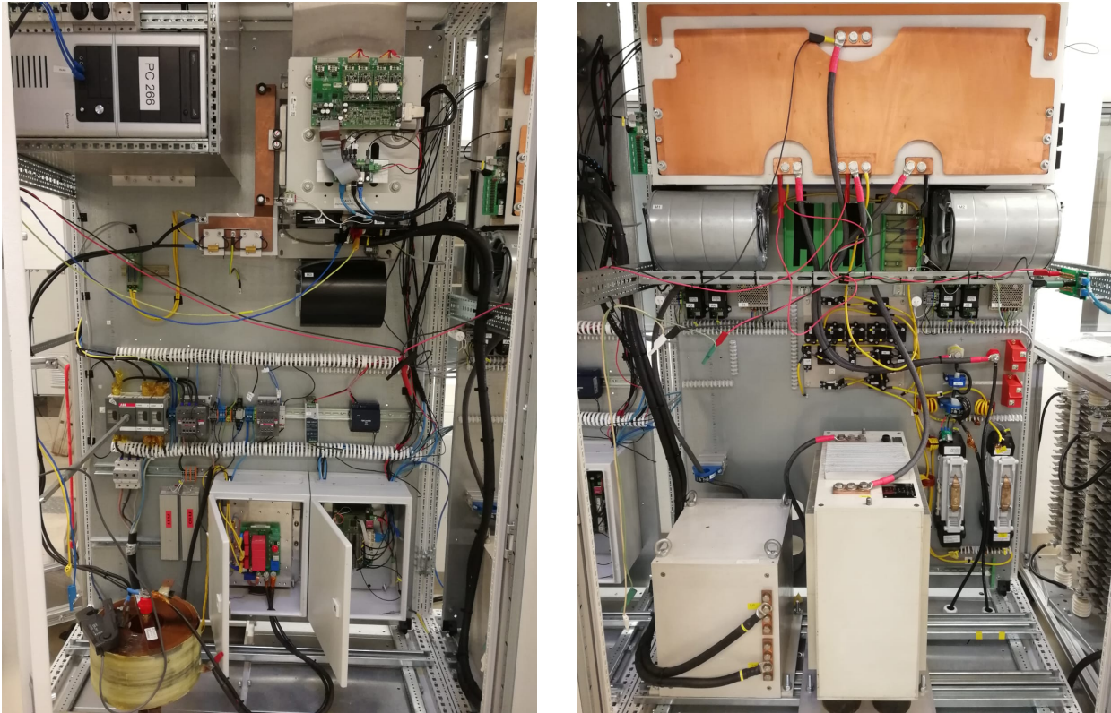
Figure 5.6: The low voltage cabinet stands on the left hand side, with the H-bridge, diode rectifier and control board, while on the right hand side, the transformer, inductance and the NPC are installed.
