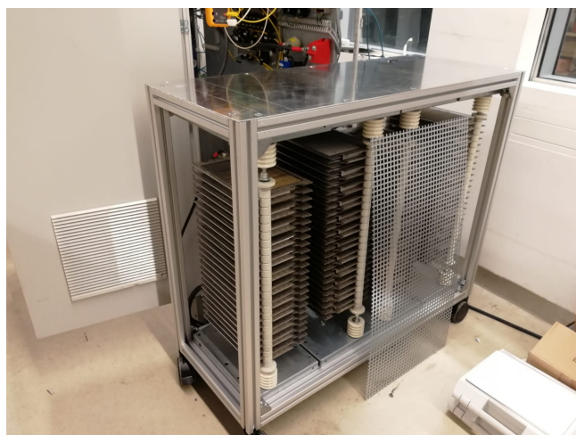
Figure 5.13: The load used during tests; four steel grid resistors of 80\Omega are connected in series.
