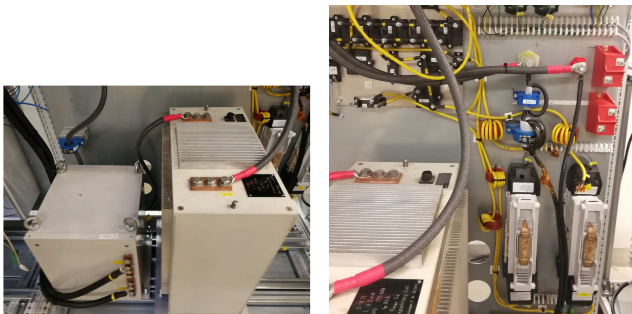
Figure 5.13: The load used during tests; four steel grid resistors of 80\Omega are connected in series.
