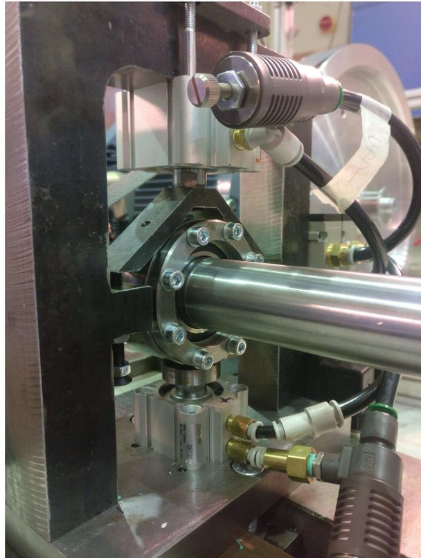
FIGURE 3.3: Holder plate assembly in the engaged position (Aalto university Paperikoneet laboratory)
