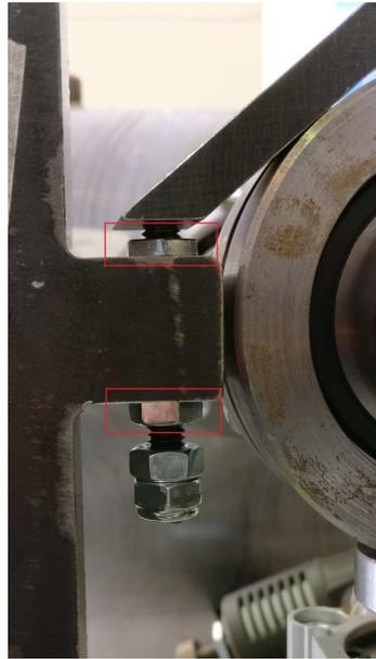
FIGURE 4.4: Detail of the positioning of the locking nuts on the positioning screws
