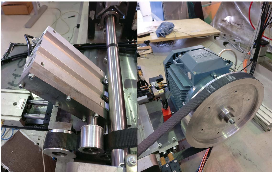
FIGURE 3.2: Belt engaging system (left) and motor assembly (right)
