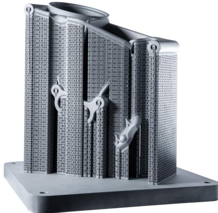
*Figure I.VII - Oerlikon AM - Oil filter housing with support structures [11]*
