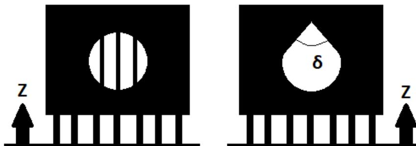
*Figure 4.2 - Vertical holes, left with support, right with drop shape.  $\delta$  is the downskin angle*
