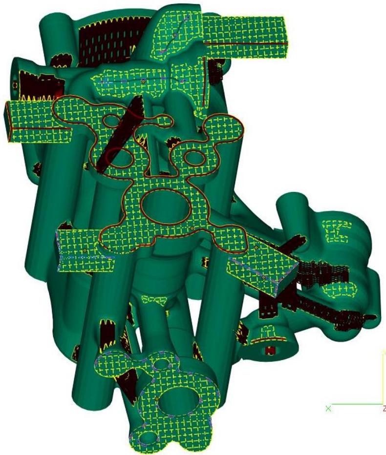
*Figure 6.7 - Support structures, bottom view, Magics*
