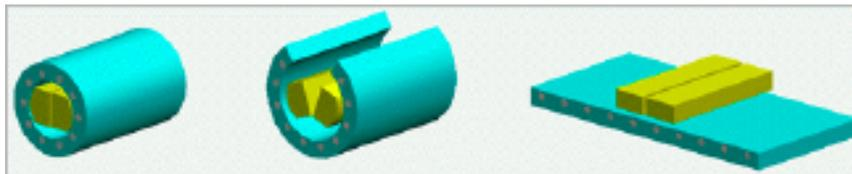
Figure 2.2: From a traditional asynchronous motor to a linear motor
