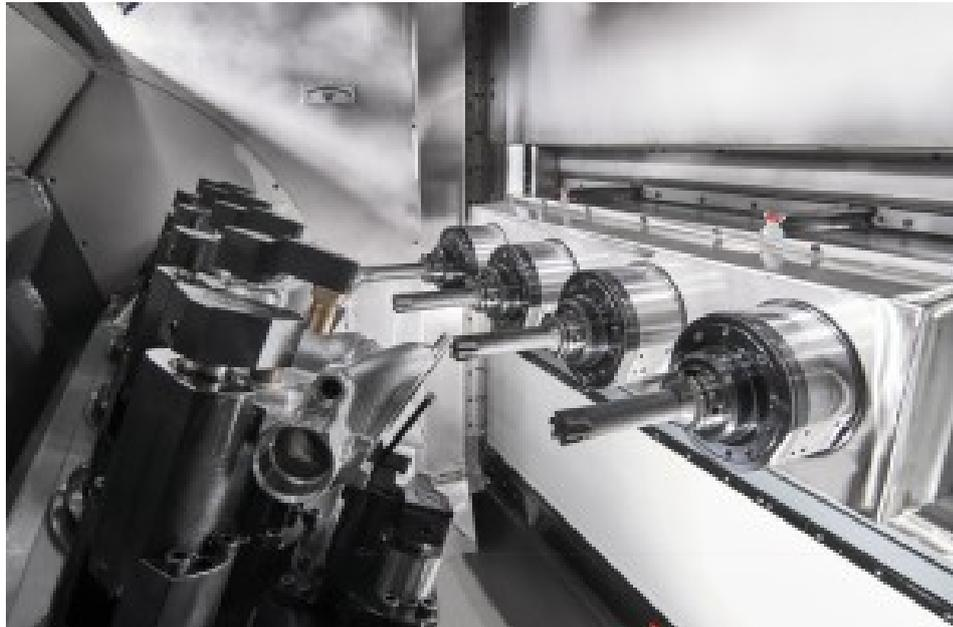
Figure 1.7: Spindles in a four working spindle configuration
