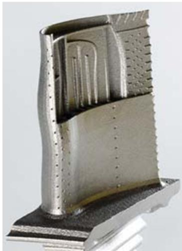
*Figura 9 - Blade cooling [16]*
