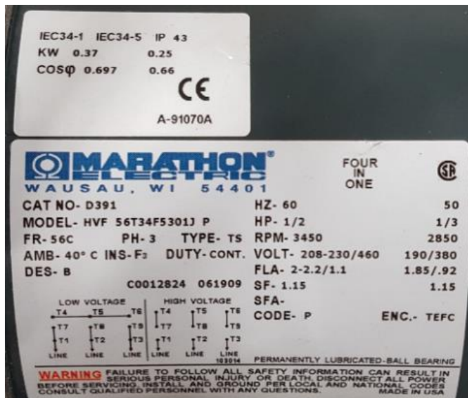
Figure 7.2-17 Electric Motor Type 3 Nameplate.
