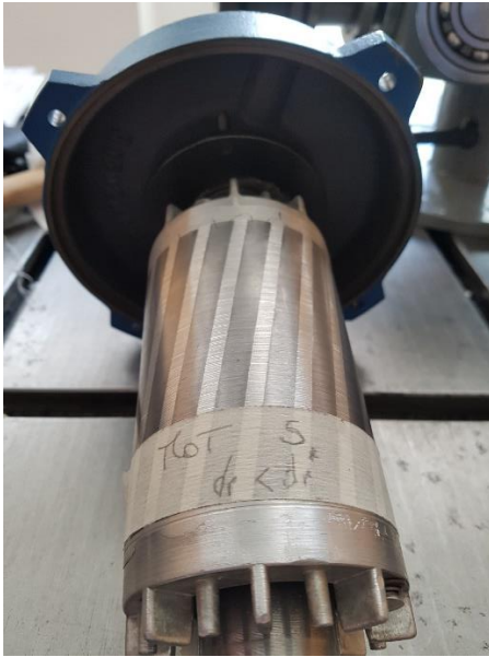
Figure 7.2-16 Grinded rotor picture for increased air gap test.
