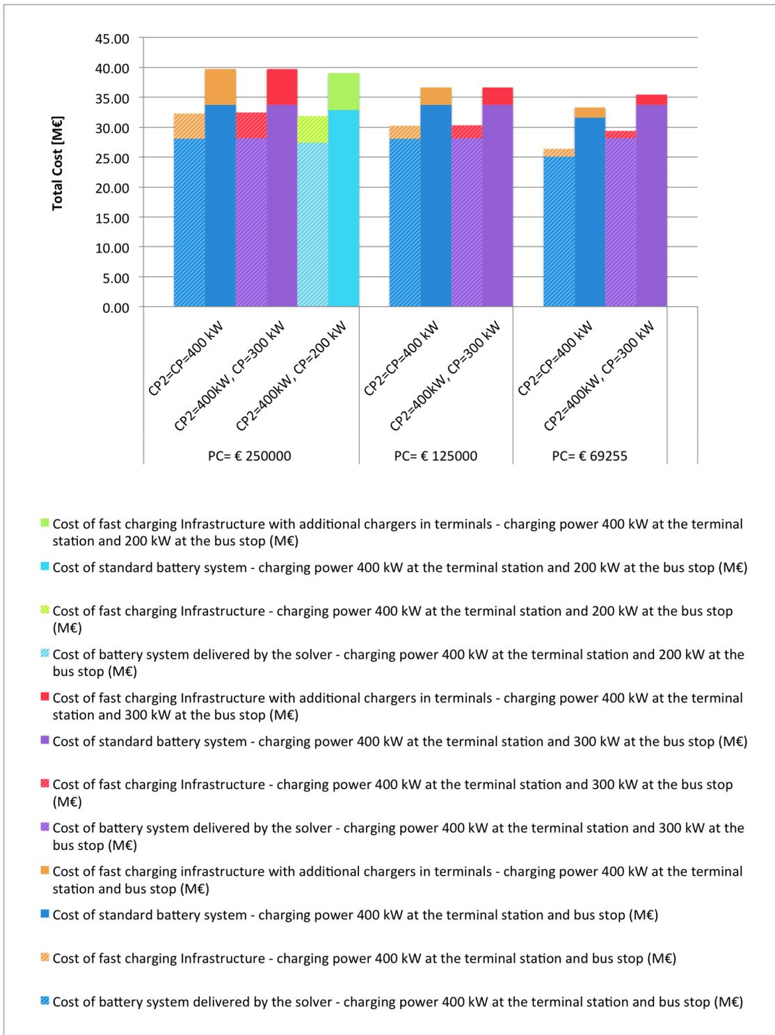
Figure 3.24 – Electrification costs with charging power of 400 kW at the terminal station
