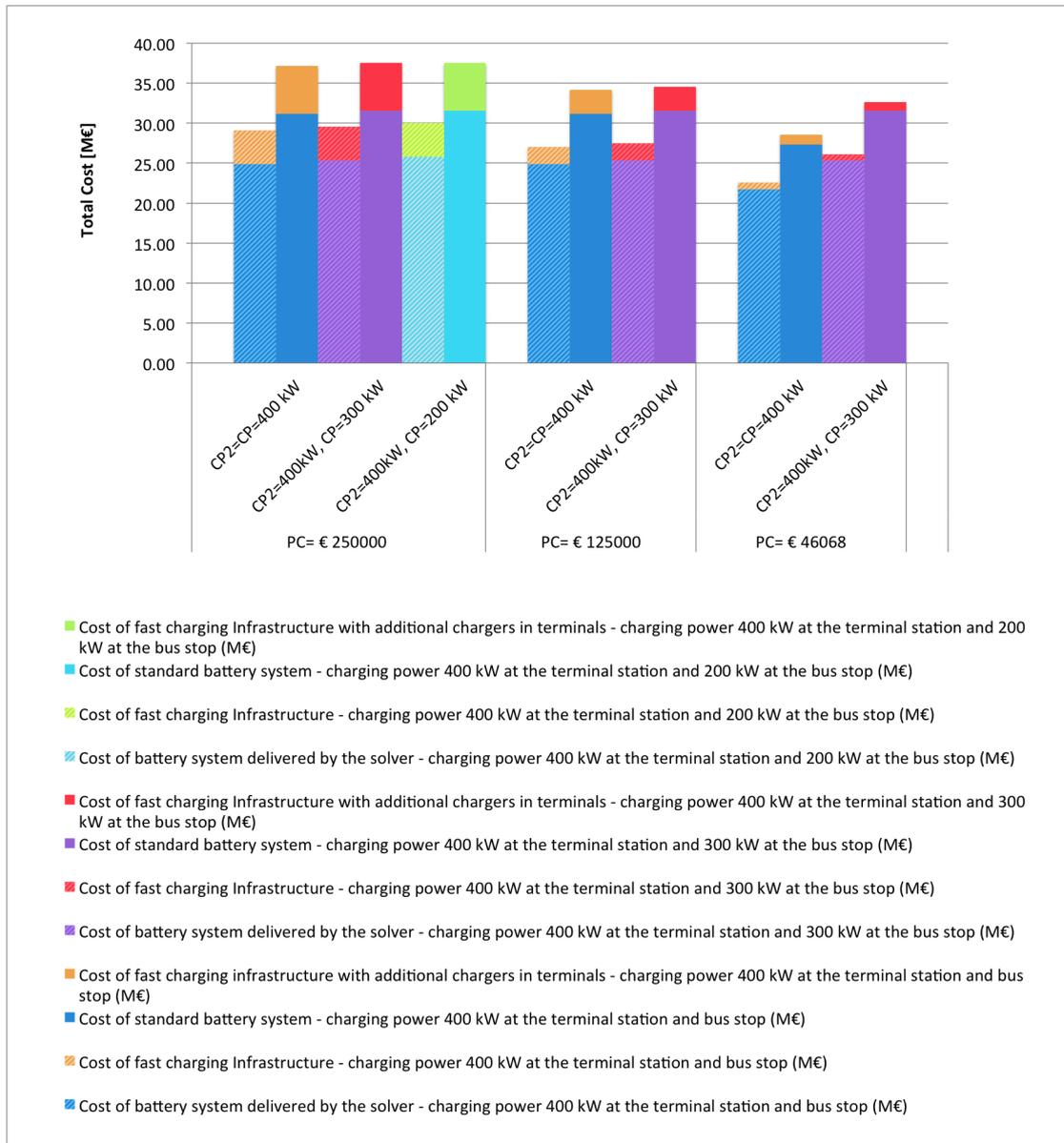
Figure 3.14 – Electrification costs with charging power of 400 kW at the terminal station
