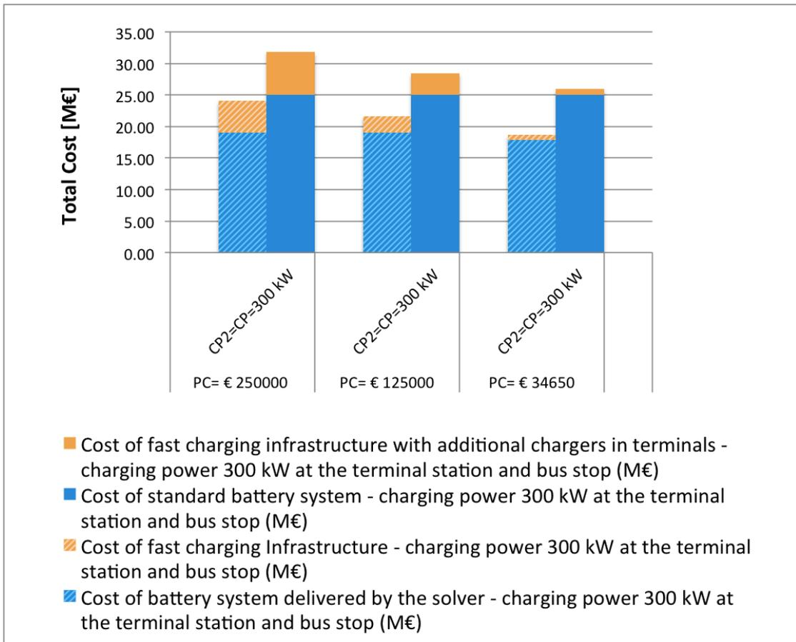
Figure 3.10 – Electrification costs with charging power lower than 400 kW at the terminal station and in bus stops
