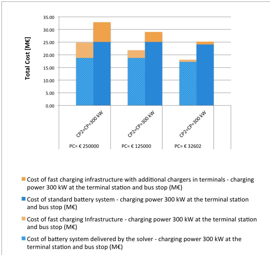
Figure 3.25 – Electrification costs with charging power lower than 400 kW at the terminal station and in bus stops
