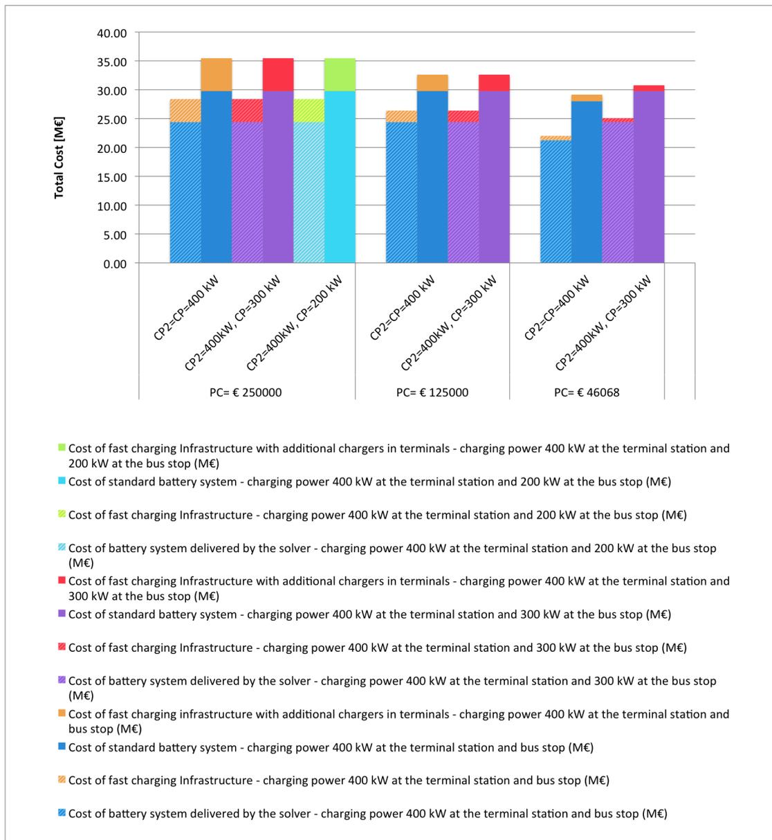
Figure 3.9 – Electrification costs with charging power of 400 kW at the terminal station
