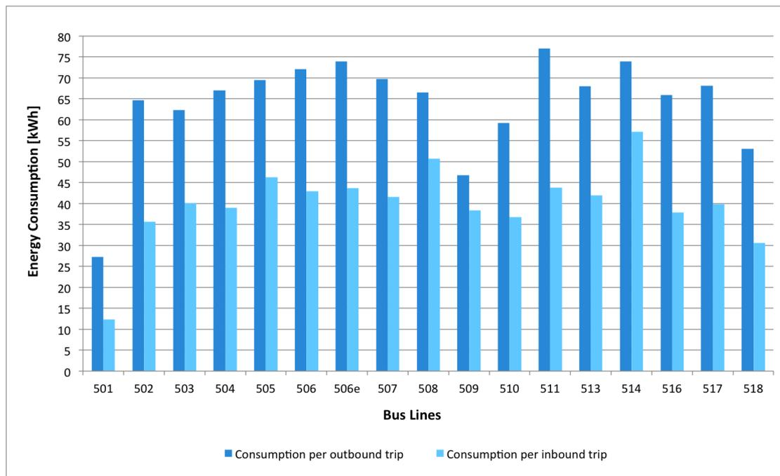
Figure 3.11 – Energy consumption per outbound trip and per inbound trip for each bus line in scenario 2
