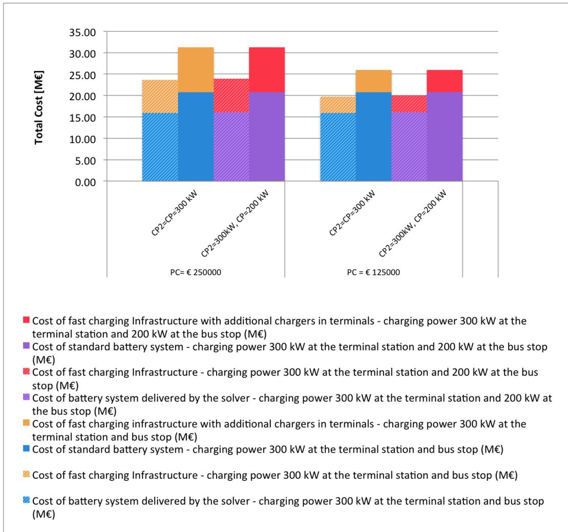
Figure 3.18 – Electrification costs with charging power lower than 400 kW at the terminal station and in bus stops
