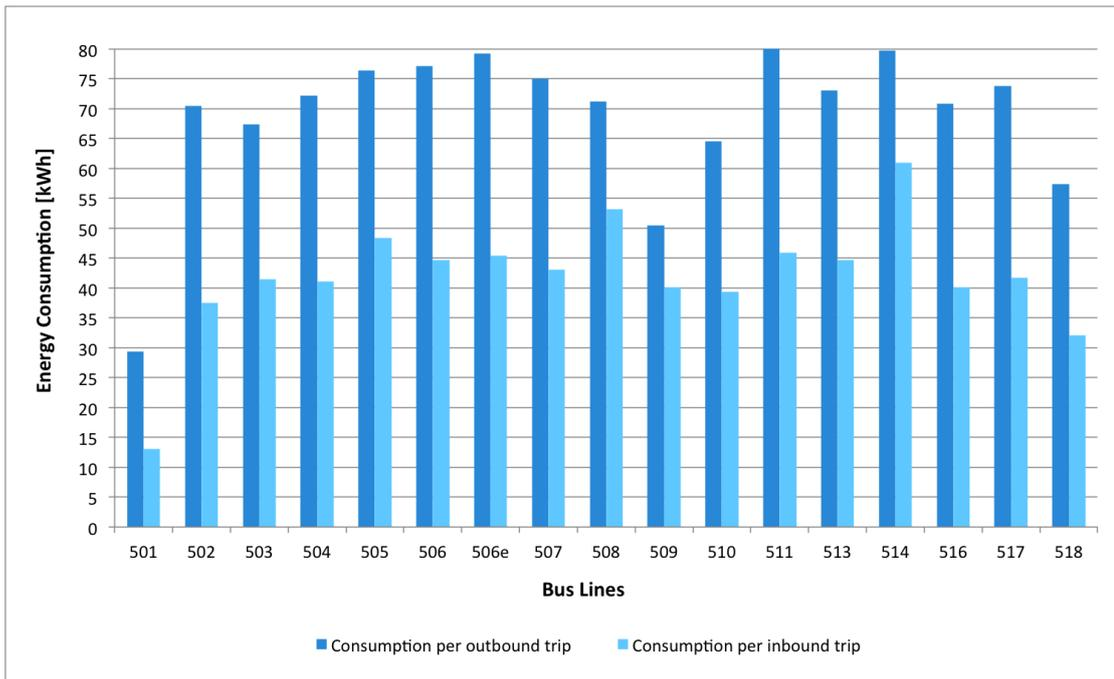
Figure 3.21 – Energy consumption per outbound trip and per inbound trip for each bus line in scenario 4
