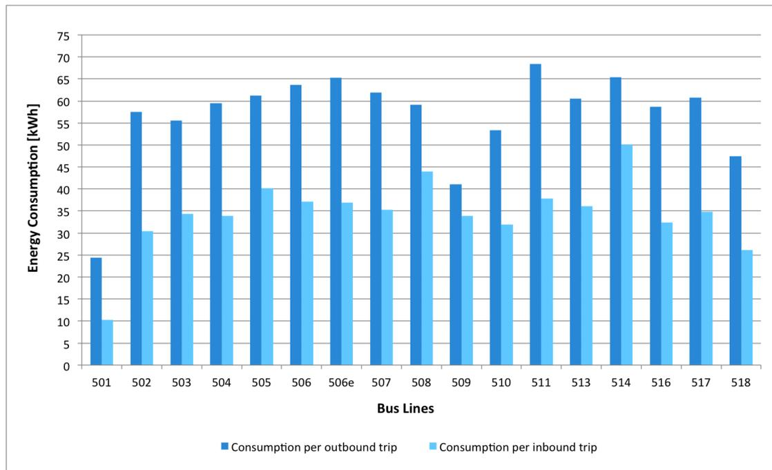
Figure 3.1 – Energy Consumption per outbound and inbound trip for each bus line in the reference case of option A
