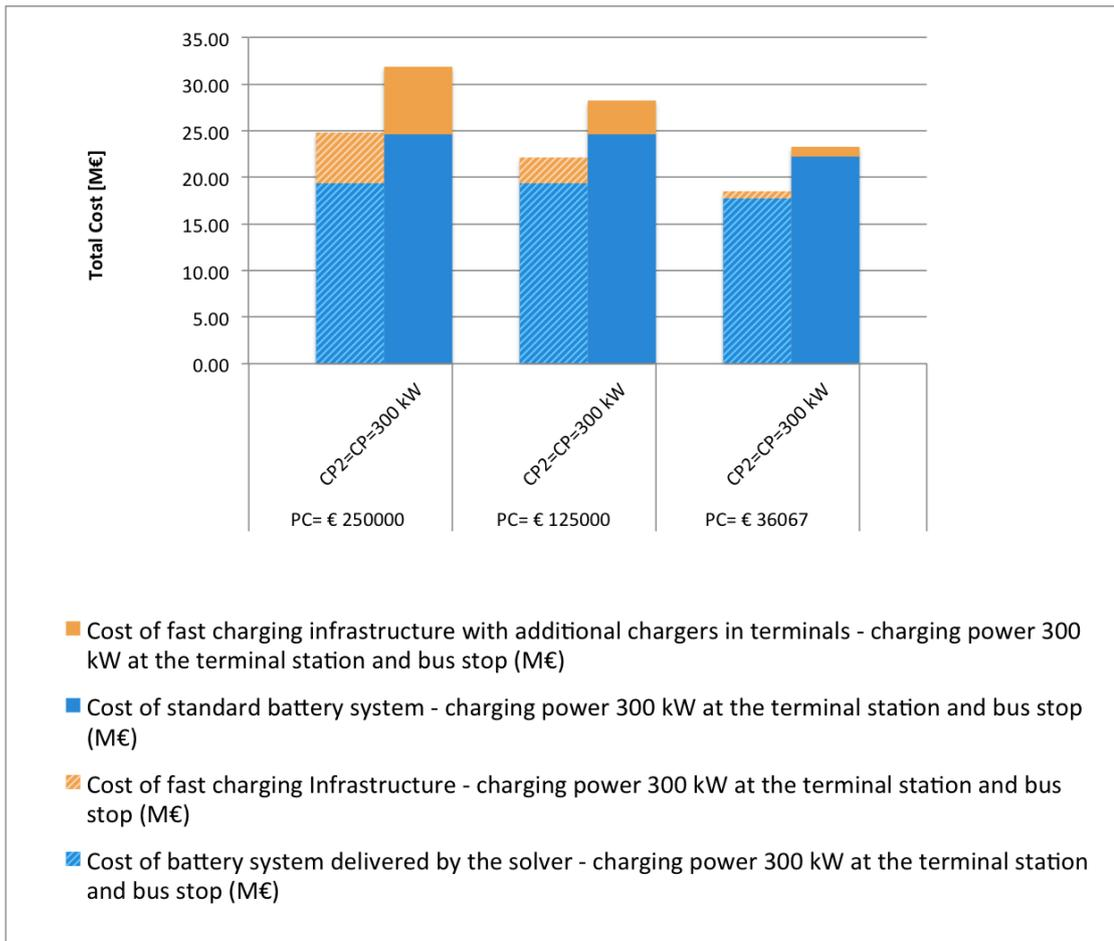
Figure 3.20 – Electrification costs with charging power lower than 400 kW at the terminal station and in bus stops
