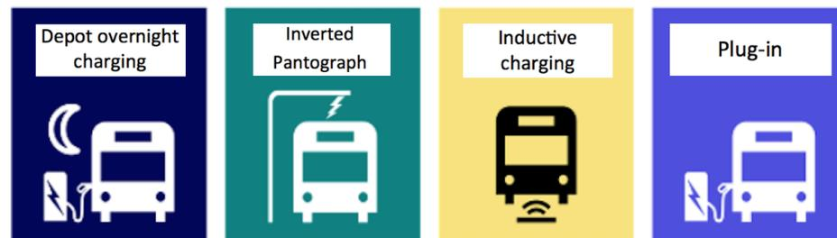
Figure 1.1 – Charging Methods: Depot overnight charging, Opportunity charging: Inverted Pantograph, Inductive Charging and Plug-in.
