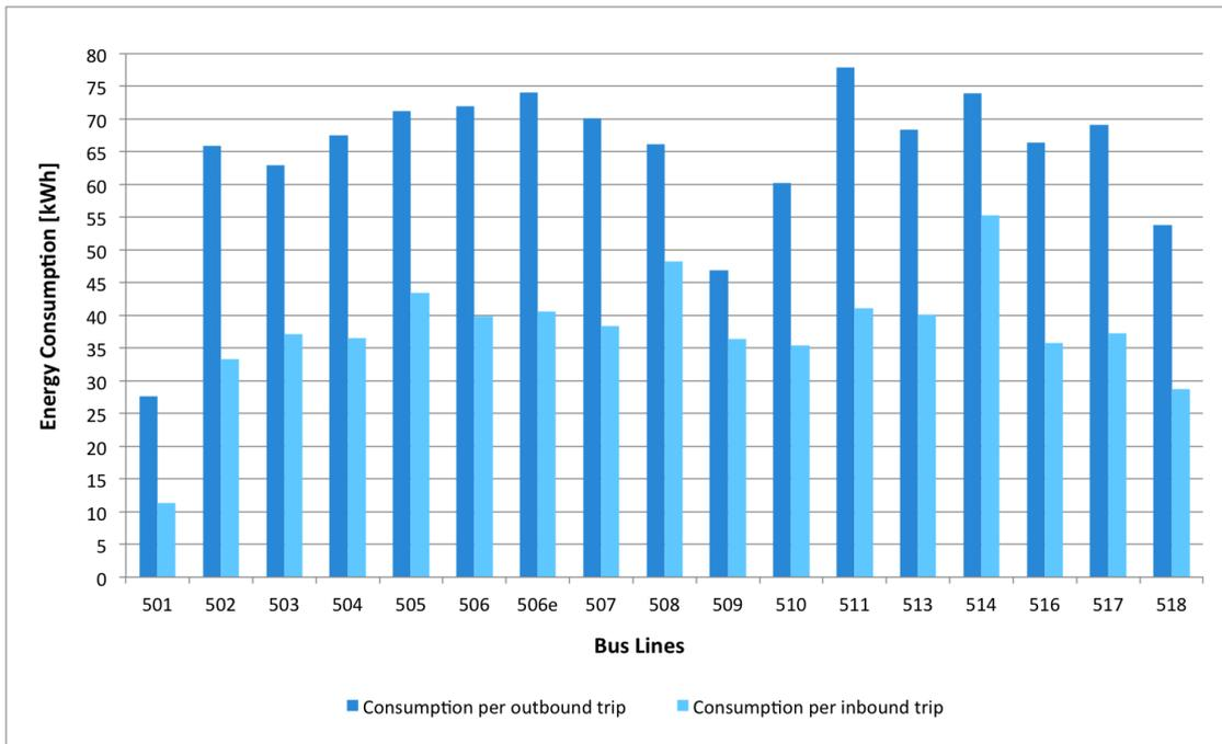
Figure 3.16 – Energy consumption per outbound trip and per inbound trip for each bus line in scenario 3
