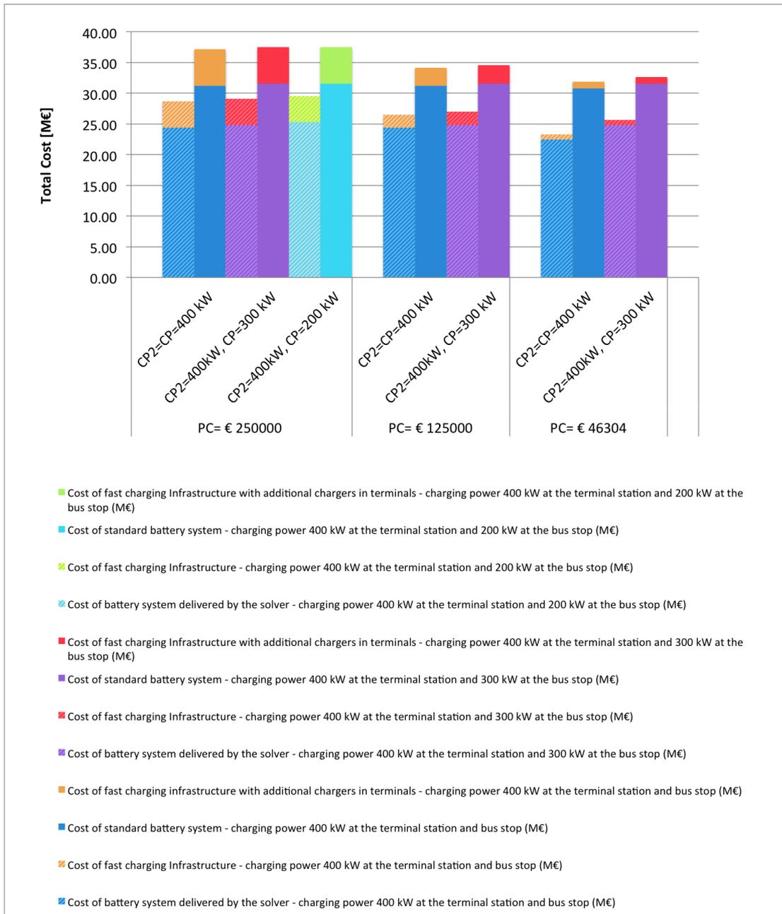
Figure 3.19 – Electrification costs with charging power of 400 kW at the terminal station
