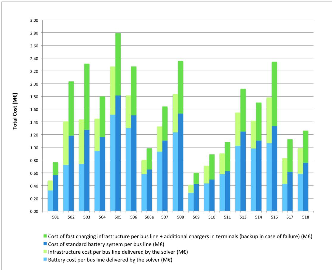
Figure 3.3 – Electrification costs per fleet and bus line for the reference case of the option A
