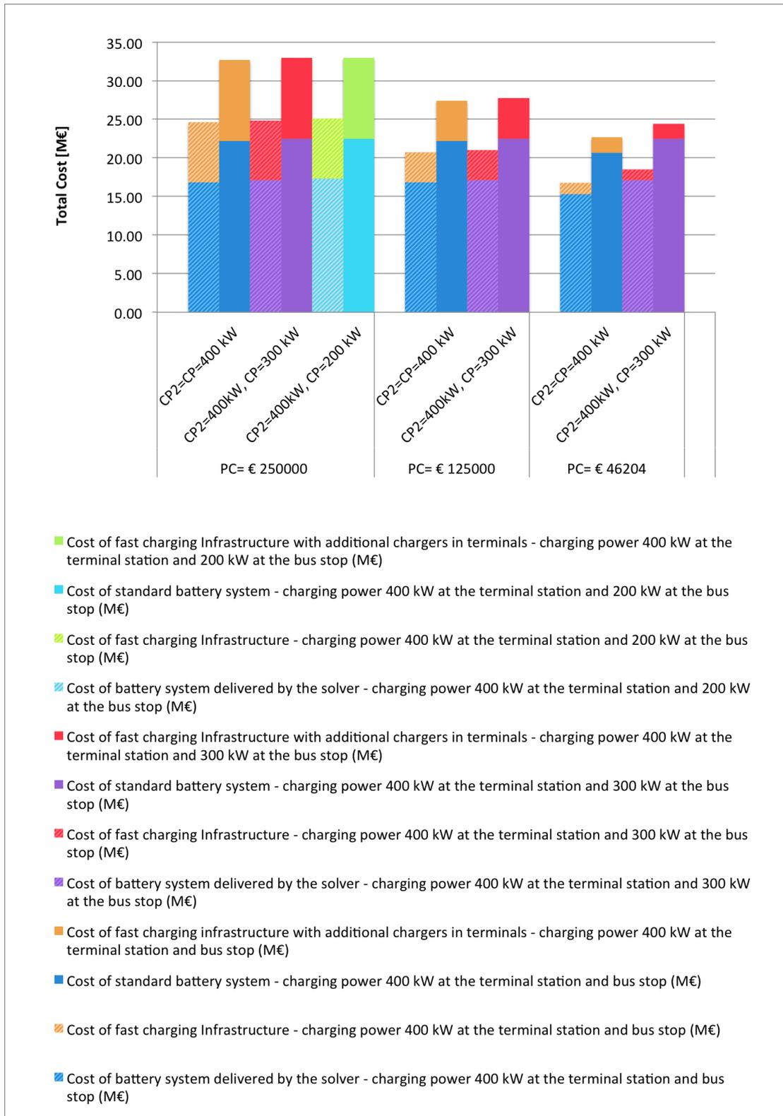
Figure 3.22 – Electrification costs with charging power of 400 kW at the terminal station
