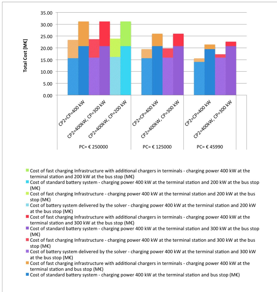
Figure 3.17 – Electrification costs with charging power of 400 kW at the terminal station
