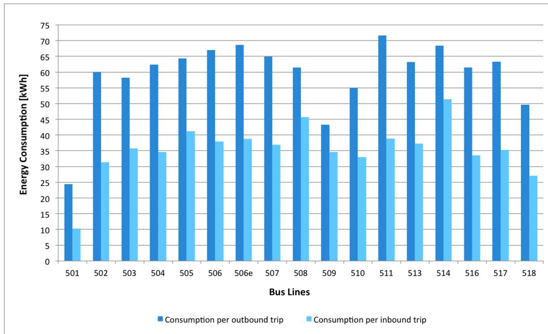
Figure 3.4 – Energy consumption per outbound and inbound trip for each bus line in the reference case of option B
