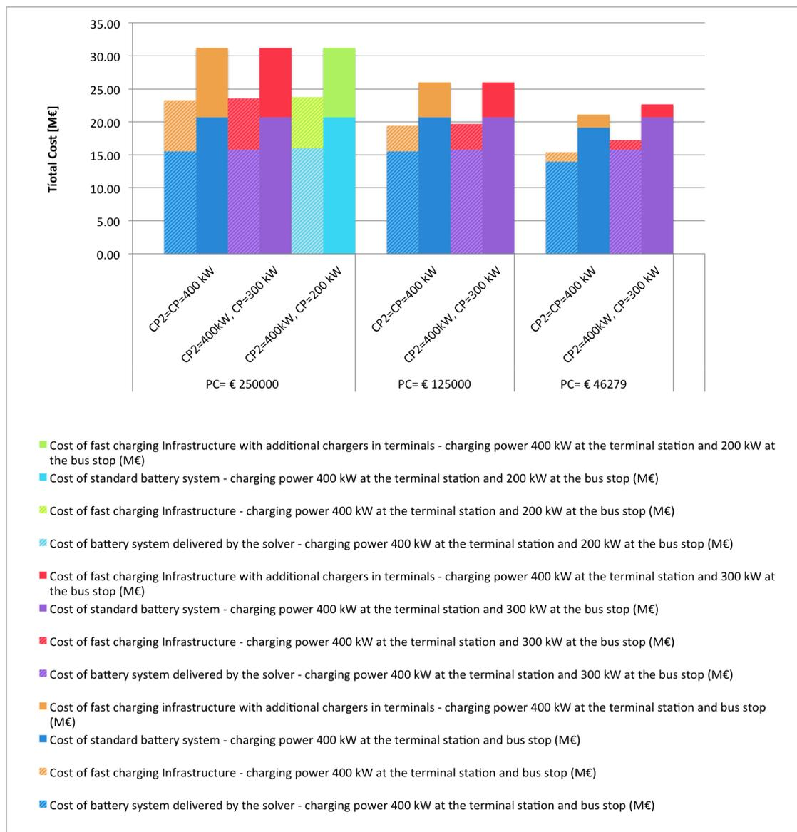
Figure 3.12 – Electrification costs with charging power of 400 kW at the terminal station
