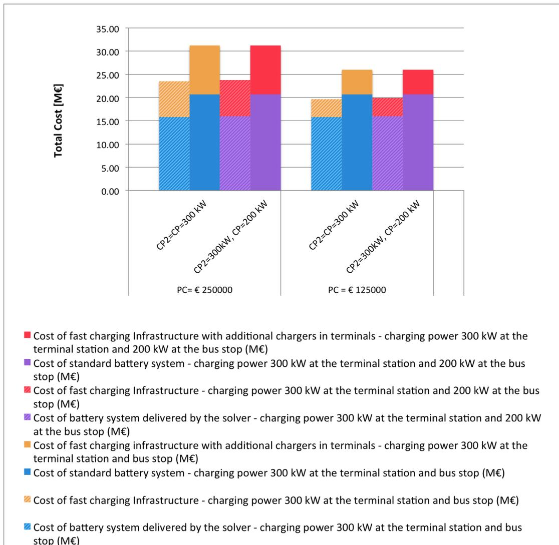
Figure 3.13 – Electrification costs with charging power lower than 400 kW at the terminal station and in bus stops
