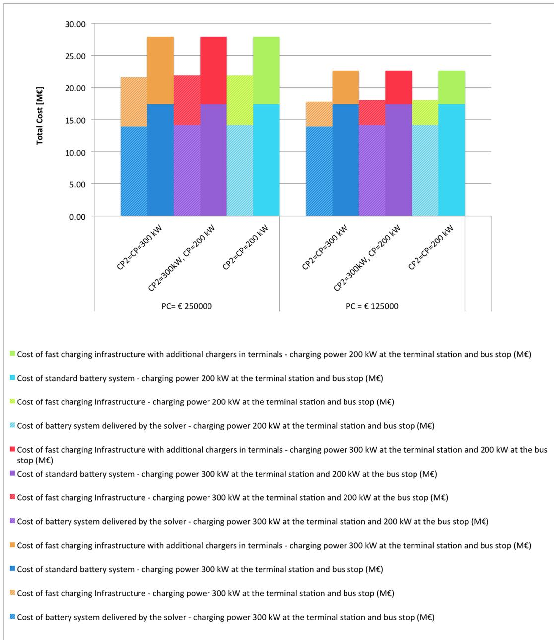
Figure 3.8 – Electrification costs with charging power lower than 400 kW at the terminal station and in bus stops
