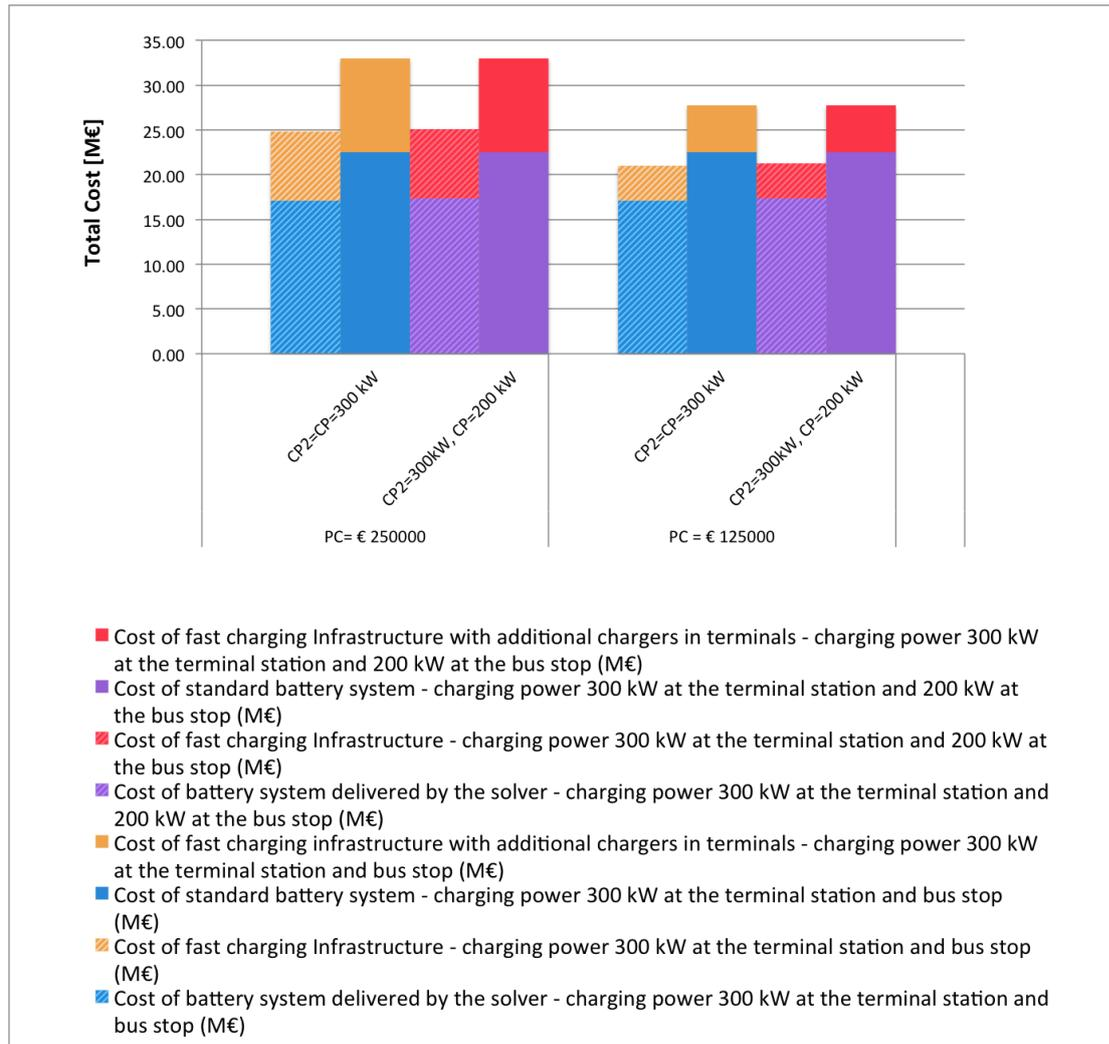
Figure 3.23 – Electrification costs with charging power lower than 400 kW at the terminal station and in bus stops
