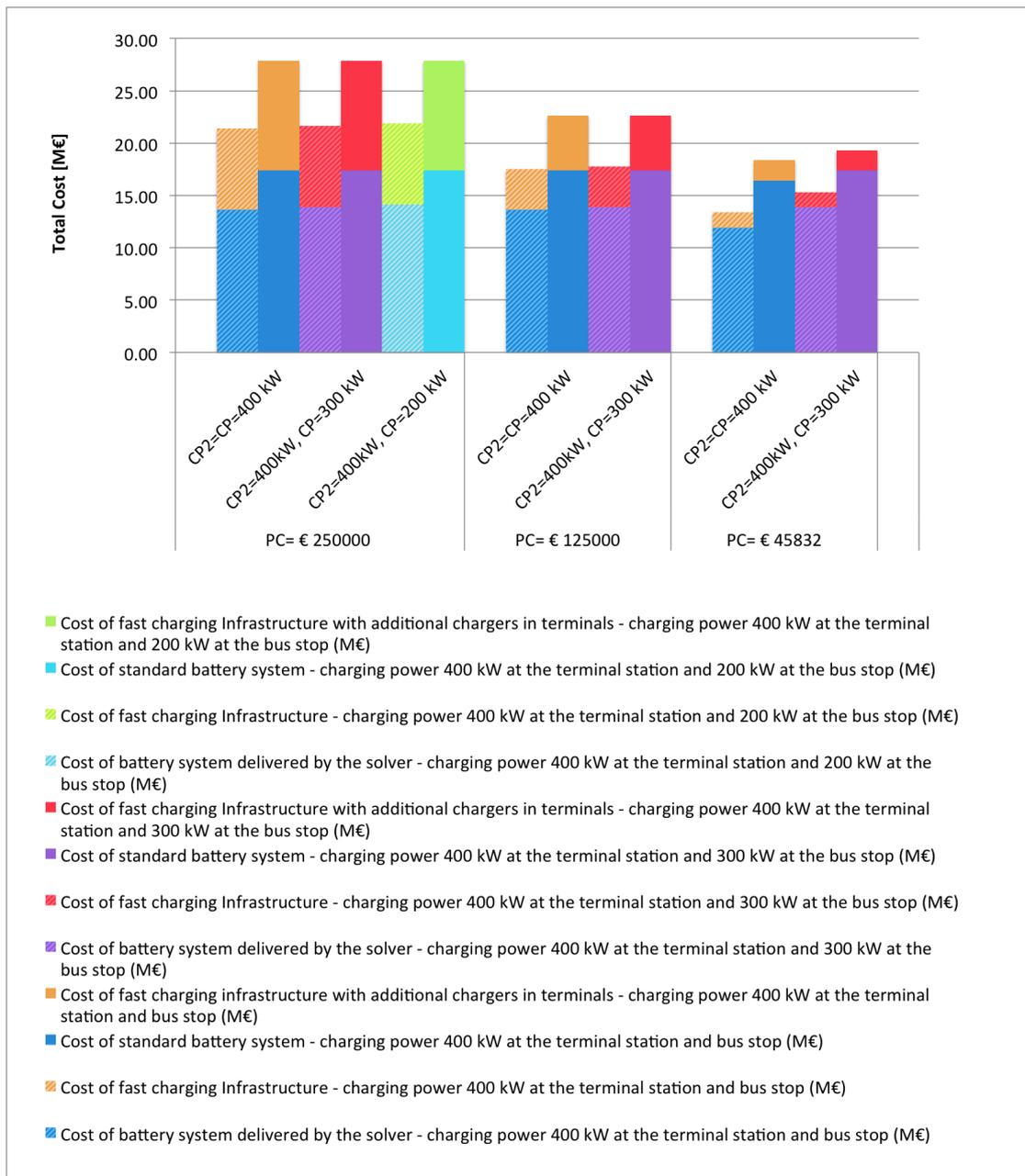
Figure 3.7 – Electrification costs with charging power of 400 kW at the terminal station
