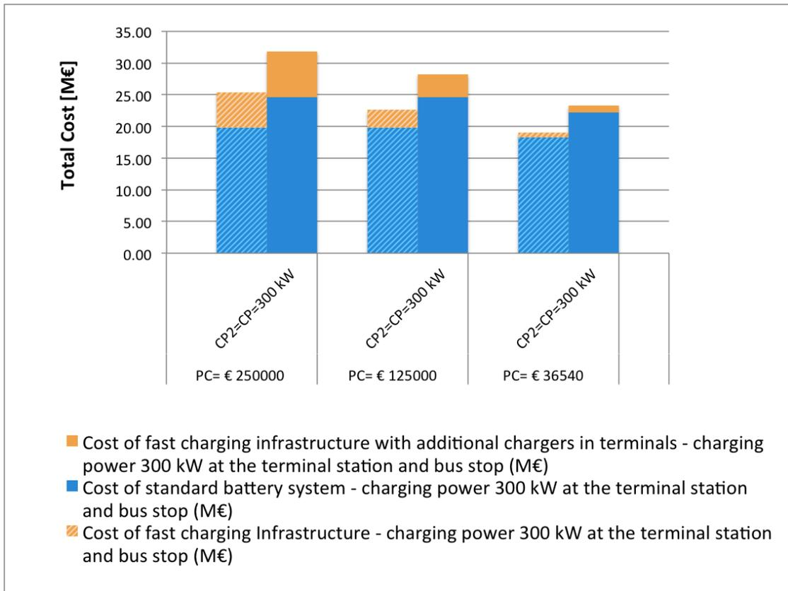
Figure 3.15 – Electrification costs with charging power lower than 400 kW at the terminal station and in bus stops
