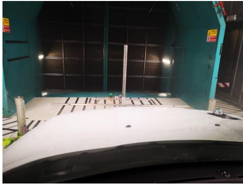
Figures 18 and 19: the windscreen a couple of seconds after turning on the wipers; on the left picture the air pressure system is 3 bar, on the right picture the air pressure system is 2 bar
