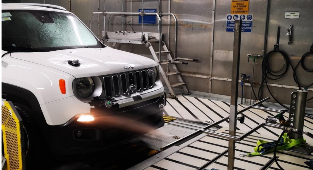
Figure 16: the spray at 3 bar of air pressure, similar to mist
