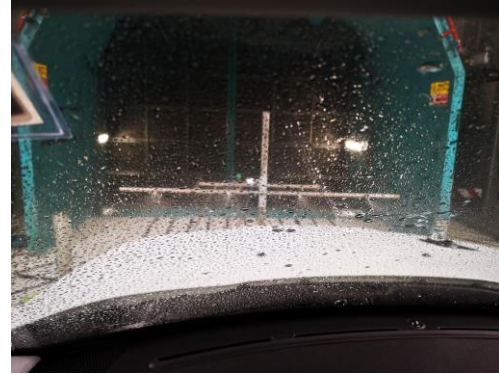
Figures 18 and 19: the windscreen a couple of seconds after turning on the wipers; on the left picture the air pressure system is 3 bar, on the right picture the air pressure system is 2 bar
