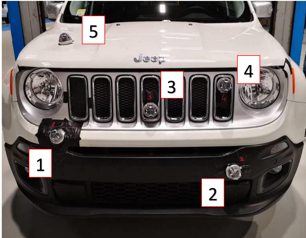
Figure 15: the layout of the sensors on the front bumper.
