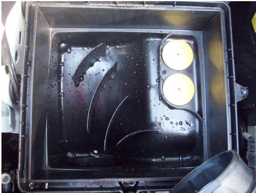
Figure 3: inspection of a filter box, clean air side, after a water ford test. The test is negative because the water passes through the filter. Note the two yellow membranes that closes the back-up holes
