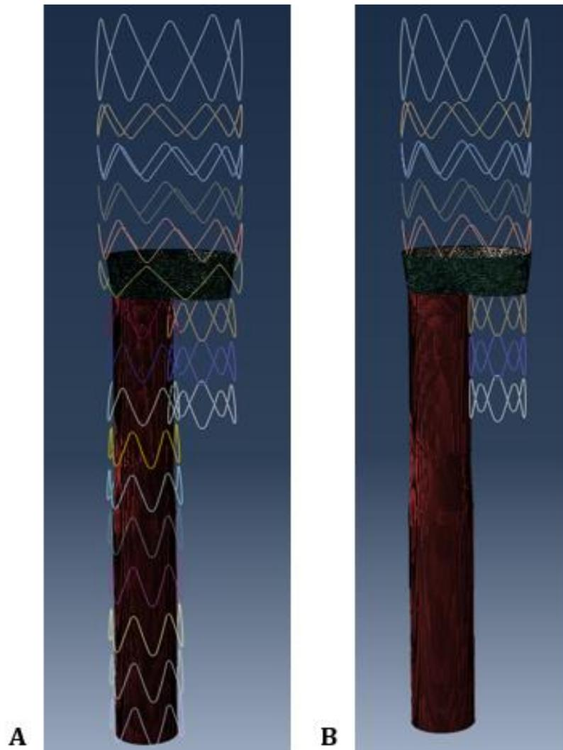
Figure 3.12: SG main body building. (A) Nitinol Stents and graft generated by Matlab input files. (B) Stent and graft crimped in Abaqus.
