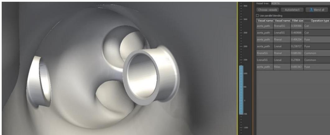
Figure 3.2: Boolean operations used (right side of the image) and a view of the interior of the aorta. In the foreground the protrusions of the stents and in the background the cavities of the two iliac arteries.
