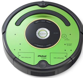
Figure 1.4: iRobot Create2 programmable robot
